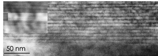
FIG. 2. Bright-field XTEM micrograph of a 20-period (In,Ga)N/GaN MQW on GaN/Al<sub>2</sub>O<sub>3</sub>. The scale is indicated. The inset shows a Fourier-filtered high-resolution micrograph of one of the wells. The (0001) lattice planes belonging to the well are highlighted.
