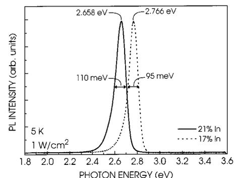
FIG. 3. PL spectra of the two 20-period (In,Ga)N/GaN MQWs on 6H-SiC(0001) and on GaN/Al<sub>2</sub>O<sub>3</sub>(0001).
