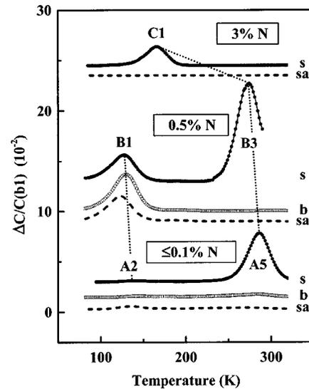
FIG. 1. Temperature scans of the DLTS signal  $\Delta C/C$  (Fourier coefficient  $b1$ ) for three Ga(As,N) compositions as indicated (0.47 s time constant, 100 ms pulse width). The deep-level spectra labeled s and sa were measured close to the surface of as-grown and annealed layers, respectively. The b scans originate from the Ga(As,N) bulk. The dominant peaks are indicated. Dotted lines connect the peaks of electron traps with similar features. Spectra are vertically shifted for clarity.
