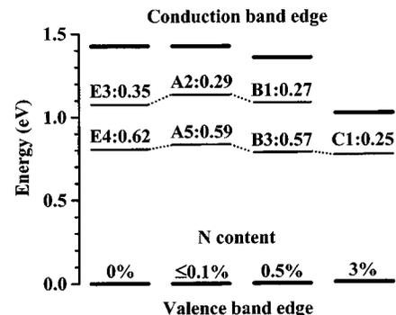
FIG. 2. Compositional dependence of dominant deep levels in the Ga(As,N) band gap. The top of the GaAs valence band is set to zero. All trap energies are given in electron volts with respect to the conduction band edge. Dotted lines connect levels of the same origin. For the traps E3 and E4, the level energies are taken from Ref. 20.
