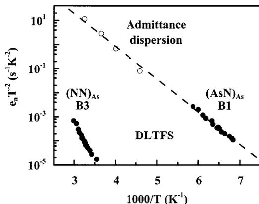
FIG. 5. Arrhenius plots of the thermal emission rate  $e_n$  for the dominant electron traps B1 [ $(AsN)_{As}$  defect] and B3 [ $(NN)_{As}$  defect] deduced from Fig. 1 for Ga(As,N) with 0.5% N (dots). The temperature dependence of  $\tau^{-1}/2$  determined from the admittance dispersion in Fig. 4 (circles) correlates with the B1 characteristics (dashed line).
