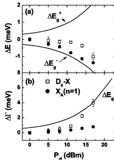
FIG. 4. Changes in (a) energy  $\Delta E$  and (b) linewidth  $\Gamma$  of the PL line from the  $X_{A,n=1}$  (dots) and  $D_0-X$  (squares) transitions as a function of the SAW rf power  $P_{rf}$ . The lines in (a) display the calculated maximum ( $\Delta E_g^+$ ) and minimum ( $\Delta E_g^-$ ) energy shifts induced by the SAW strain near the sample surface. The line in (b) shows the peak-to-peak modulation of the band gap  $\Delta E_g = \Delta E_g^+ - \Delta E_g^-$ .
