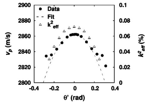
FIG. 2. Phase velocity  $v_p$  of the surface-acoustic wave (circles, from Ref. 30) and calculated effective electromechanical coupling  $k_{eff}^2$  (triangles) as a function of the deviation angle  $\theta'$  from the  $[0\bar{1}1]$  direction. The dashed line is a fit to the parabolic dispersion given by Eq. (1).
