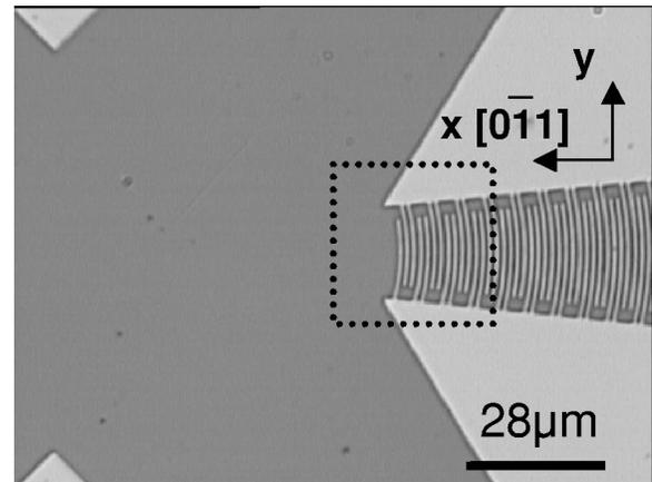
FIG. 4. Optical micrograph of the aperture output of a double-finger focusing transducer ( $DF_2$  in Table I). The curved fingers are designed to follow the group velocity curves. The two triangles at the upper and lower corners indicate the origin  $O$  (cf. Fig. 1). The dotted rectangle indicates the area scanned in the interferometry measurement shown in Fig. 5.
