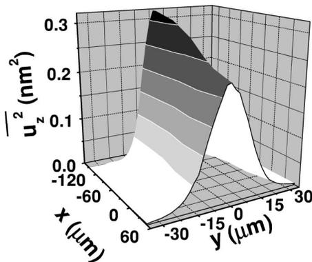
FIG. 6. Two-dimensional profile of the square of the vertical displacement field averaged over time ( $\overline{u_z^2}$ ) measured in front of double-finger interdigital transducer  $DF_1$  (powered with  $P_{rf}=10$  mW). The position  $(x,y) = (0,0)$  corresponds to the origin  $O$  (cf. Fig. 1).
