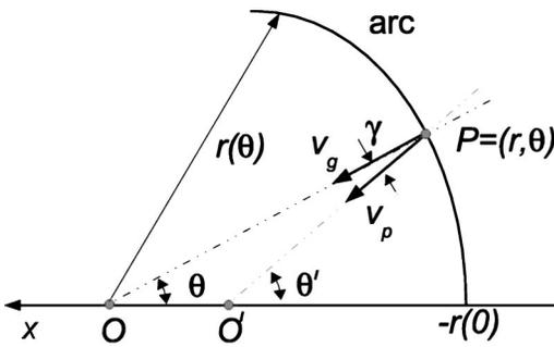
FIG. 1. Scheme of focusing of a surface-acoustic wave by an arc-shaped interdigital transducer finger. *O* denotes the focus position,  $\theta$  and  $\theta'$  are the propagation directions of the group ( $v_g$ ) and phase velocity ( $v_p$ ), respectively.
