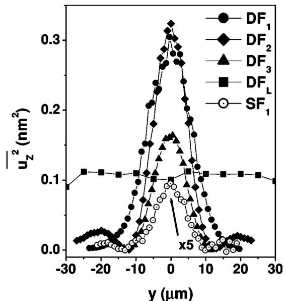
FIG. 8. Profile of the square of the vertical displacement field averaged over time ( $\overline{u_z^2}$ ) along the beam cross section measured by interferometry in front of different focusing interdigital transducers of set 1. The profile for single-finger interdigital transducer  $SF_1$  is also displayed for comparison.
