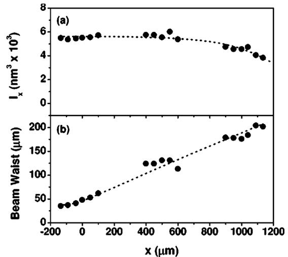
FIG. 7. (a) Integrated power flux  $I_x = \int_{-\infty}^{\infty} \overline{u_z^2}(x,y) dy$  through the beam cross section and (b) beam waist  $w_b$  as a function of the distance from the focus for double-finger interdigital transducer  $DF_1$ . The position  $x=0$  corresponds to the origin  $O$ .
