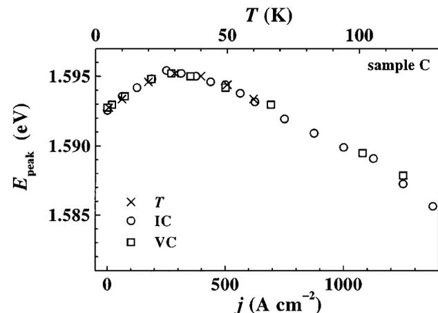
FIG. 10. PL peak energy  $E_{\text{peak}}$  in sample C versus current density  $j$  at  $T=5 \text{ K}$  for voltage-controlled (squares) as well as current-controlled (circles) measurements and versus sample temperature  $T$  (crosses) at zero bias. The horizontal scales have been adjusted relative to each other to clearly show the agreement of the effect of these two parameters.
