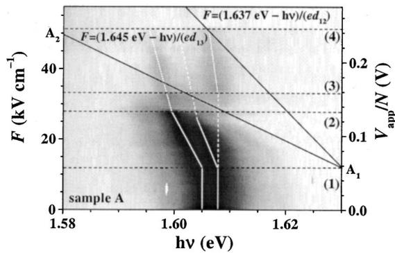
FIG. 2. Gray-scale representation of the logarithm of the PL intensity of sample A versus photon energy  $h\nu$  and electric-field strength  $F$  recorded at  $T=5$  K. The excitation energy was 1.968 eV and the power 0.15 mW. The white lines following the PL peak(s) are guides to the eyes. The black lines indicate the field dependence of the spatially indirect transitions between the electrons in wells 2 and 3 with holes in the widest well 1.
