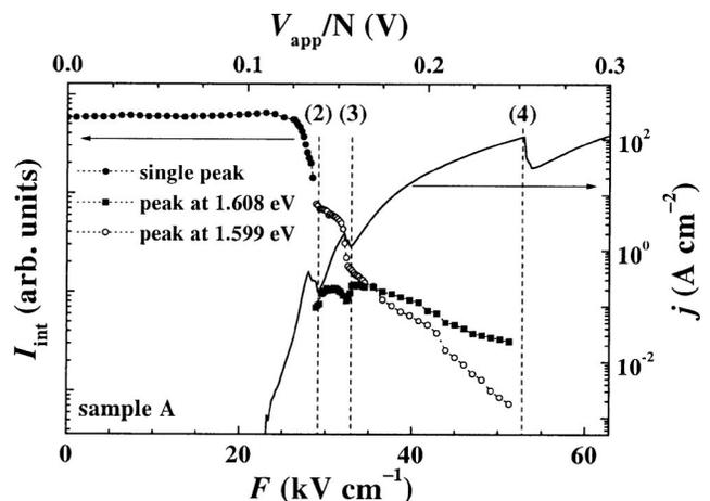
FIG. 4. Comparison between the field dependence of the logarithm of the integrated PL intensity  $I_{\text{int}}$  from the widest QW and the dark current density  $j$  of sample A. The sample is at  $T=5$  K and photoexcited at 1.70 eV with a power of 1  $\mu\text{W}$ .
