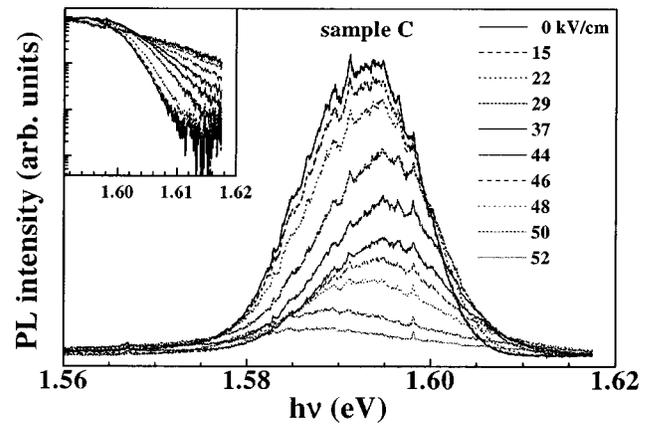
FIG. 9. PL spectra from sample C for various applied electric fields recorded at  $T=5 \text{ K}$ . The inset shows the intensity of the high-energy tail of the PL line on a logarithmic scale.
