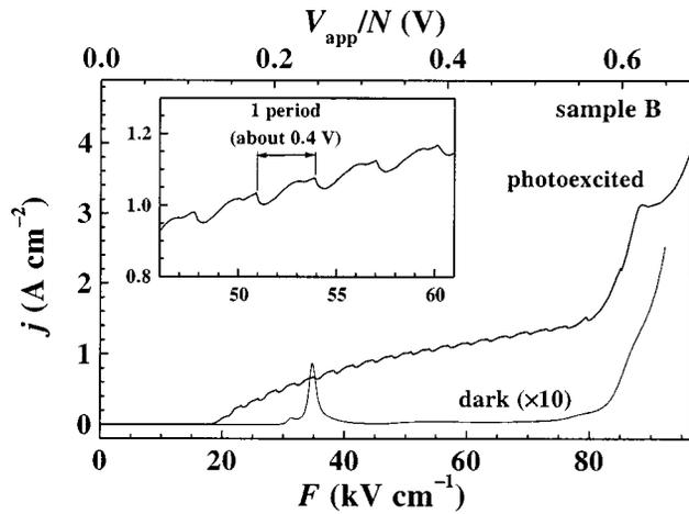
FIG. 5. Dark and photoexcited  $j$ - $F$  characteristics of sample B for an excitation energy of 1.63 eV, laser power of approximately 50 mW, and temperature  $T=5$  K. The inset shows an enlarged section of the photoexcited  $j$ - $F$  characteristics.
