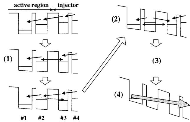
FIG. 11. Schematic diagrams for the carrier redistribution process in the quasi-QCL structure.
