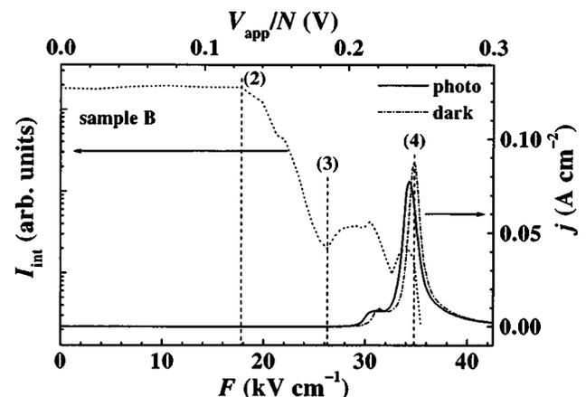
FIG. 7. Comparison between the field dependence of the logarithm of the integrated PL intensity  $I_{\text{int}}$  from the widest QW detected at approximately 1.628 eV and the current density  $j$  of sample B at  $T=5$  K. The sample is excited at 1.746 eV with a power of  $0.1 \mu\text{W}$ .
