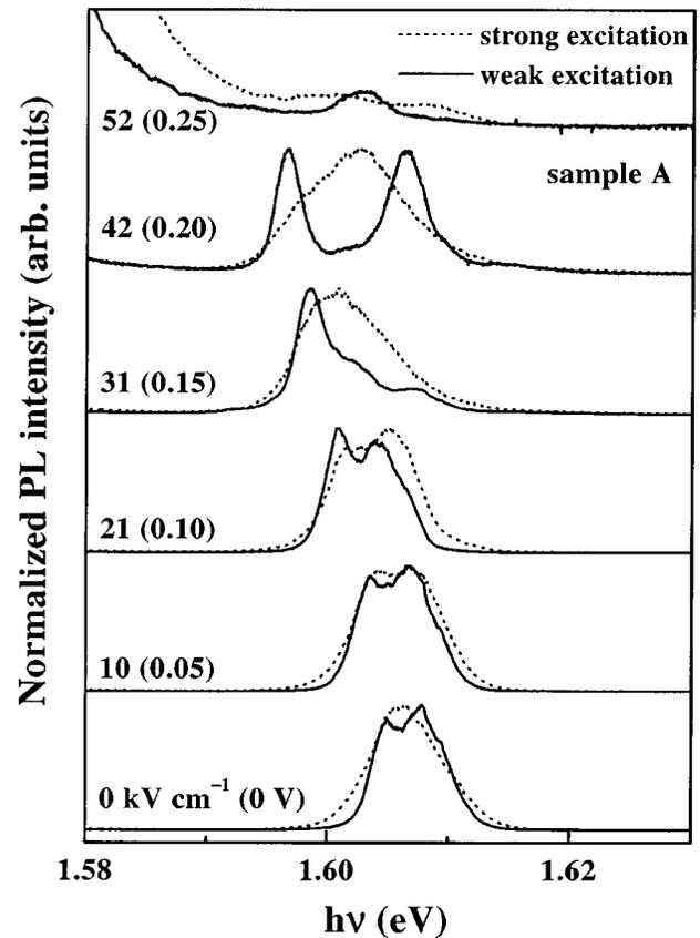
FIG. 3. Comparison of the normalized PL spectra of sample A for weak (0.5  $\mu\text{W}$ ) and strong (150 mW) excitation at a photon energy of 1.746 eV for different electric-field strengths (voltages per period) at  $T=5$  K.
