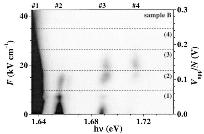
FIG. 6. Gray-scale representation of the PL intensity in sample B versus excitation photon energy  $h\nu$  and electric-field strength  $F$  for photoexcitation at 1.968 eV with a power of 15 mW recorded at  $T=5$  K. The numbers on top identify the different wells.
