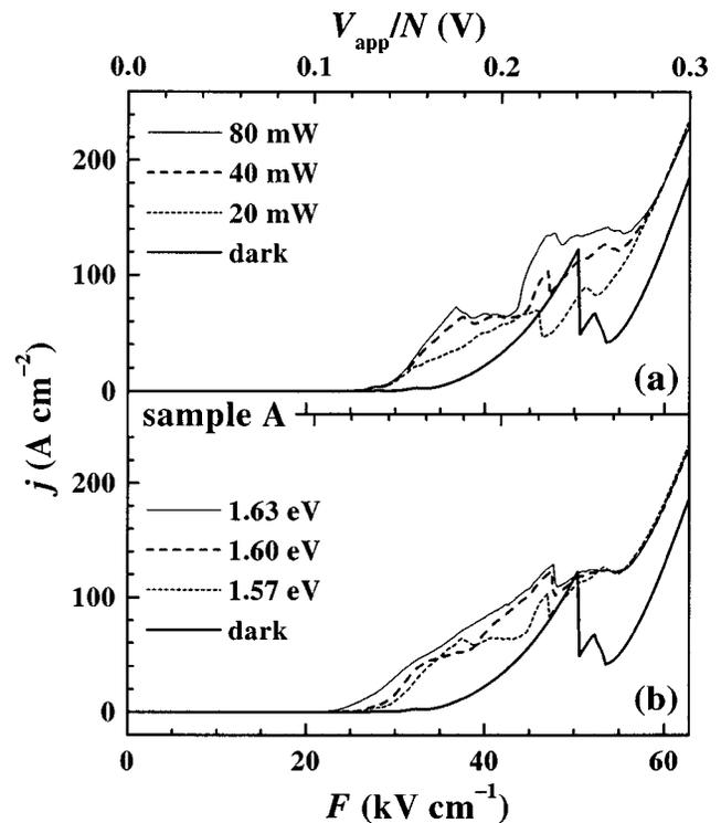
FIG. 1.  $j$ - $F$  characteristics of sample A (a) in the dark as well as for different light intensities with a photon energy of 1.57 eV and (b) for different photon energies at an intensity of 40 mW. All curves were recorded at a sample temperature  $T=5$  K.
