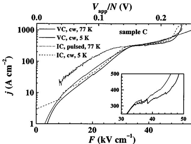
FIG. 8. Logarithm of the current density  $j$  versus field strength  $F$  of sample C. VC and IC denote voltage- and current-controlled operation, respectively. The pulsed measurement was performed using a frequency of 2 kHz and a duty cycle of 0.2%. The inset shows an enlarged section of the plateau region for the voltage-controlled measurements on a linear scale.
