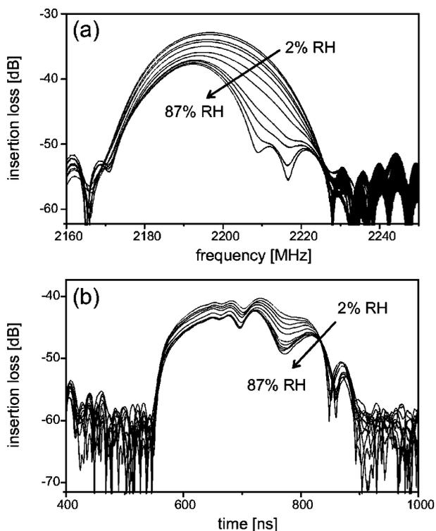
FIG. 3. Humidity dependence of the transmission curve at 2.203 GHz ( $f_{21}^1$ ) in the (a) frequency and (b) time domains.
