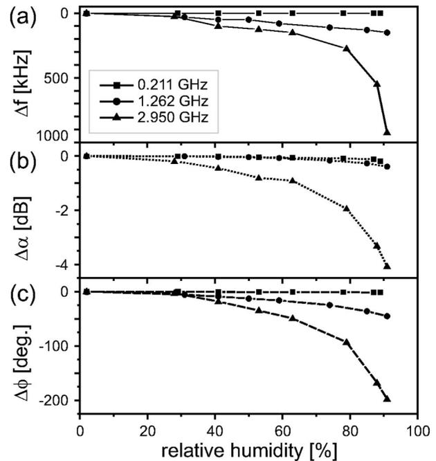
FIG. 2. Humidity dependence of selected peaks at  $f=0.211$  (I.2), 1.262 (I.12), and 2.950 GHz (I.28). Frequency shift  $\Delta f$ , attenuation  $\Delta\alpha$ , and phase shift  $\Delta\phi$  as a function of the RH.
