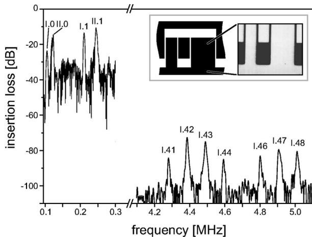
FIG. 1. SAW sensor device: A NG-FEUDT transducer is employed for efficient excitation of higher harmonics of two acoustic modes, as shown in the electrical transmission spectrum. The superscript (I/II) denotes the type of mode and the subscript ( $n=1, \dots$ ) the order of harmonic excitation. The geometry of the NG-FEUDT structure (sketch and optical micrograph shown in the inset) is repeated 20 times ( $\lambda=35 \mu\text{m}$ ). The device was fabricated by standard photolithography.
