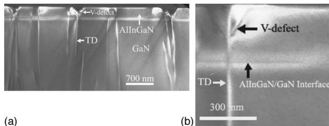
FIG. 2. (a)  $(10\bar{1}2)$  cross-section TEM image of the AlInGaN/GaN epilayer with 7% In, which is typically also observed in the other samples. (b) TEM image with a larger magnification containing a V-defect. TD denotes the threading dislocations.
