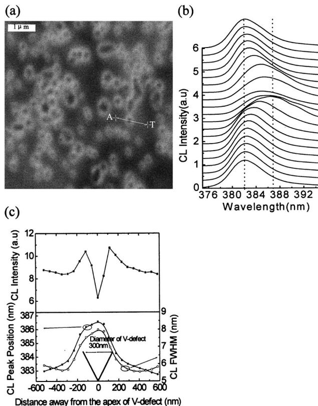
FIG. 3. (a) CL image for the AlInGaIn epilayer with an In mole fraction of 0.07 measured at 11 K and at the wavelength of 384 nm. (b) A series of 20 CL spectra obtained along a line across the V-defect as shown by the bright dotted line in (a). The distance between A and T amounts to  $1.1 \mu\text{m}$ . (c) The peak wavelength, FWHM, and integrated intensity of the CL spectra along the scanned line. The profile of the V-defect is also schematically shown in the figure.
