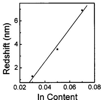
FIG. 4. The total redshift of the CL spectra as a function of the In mole fraction in different AlInGaN samples.
