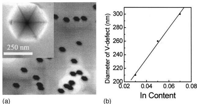
FIG. 1. (a)  $3 \times 3 \mu\text{m}^2$  AFM image of the AlInGaIn epilayer sample with an In mole fraction of 0.07. The inset shows a SEM image of a V-defect. (b) Diameter of the V-defect as a function of the In mole fraction in AlInGaIn alloy samples.
