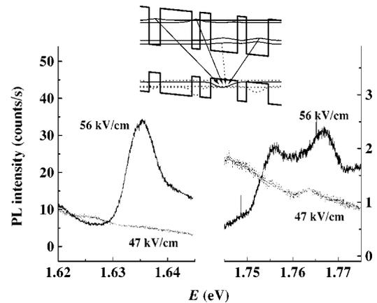
FIG. 3. PL spectra of the lower (left) and upper (right) laser levels below (47 kV/cm) and above (56 kV/cm) the critical field strength. The inset presents a schematic view of the interband PL transitions relevant for QCLs at the operation field strengths.
