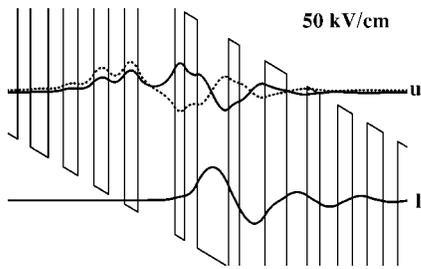
FIG. 1. Calculated envelope functions for the bonding and antibonding states of the coupled injector and upper laser levels ( $u$ , solid and dashed line, respectively) and the lower laser level ( $l$ ) at the critical field strength  $F_{\text{crit}} = 50$  kV/cm. The calculated energy separation between the bonding and antibonding states is about 3 meV.
