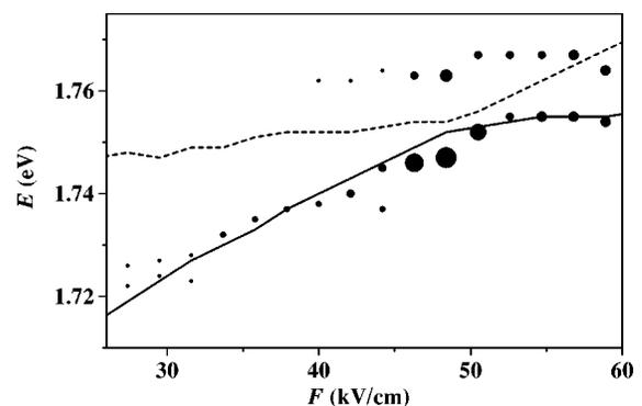
FIG. 4. Transition energies for the upper laser level and the injector state for recombination into the valence ground state as a function of electric field strength (symbols). The size of the symbols approximately represents the intensity normalized by the intensity of the ground-state transition at about 1.60 eV. For comparison, the calculated values are added (lines).
