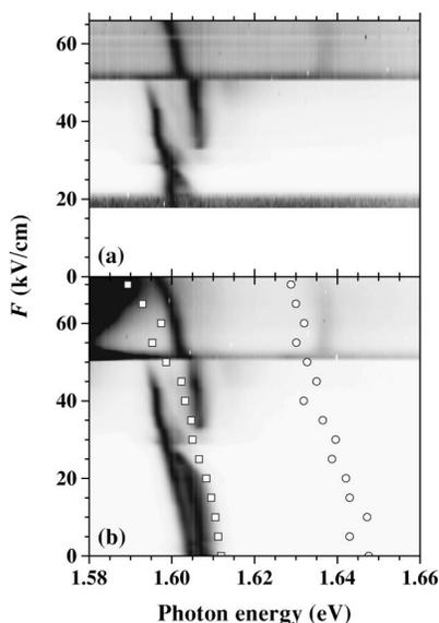
FIG. 2. Normalized, electric-field-dependent PL spectra of the conduction band ground state and the lower laser level below as well as above the critical field strength for both, (a) the anti-Stokes and (b) the Stokes configuration, in a gray-scale representation. For comparison, the calculated transition energies are added (symbols). The splitting of the PL line of the ground state for  $30$  kV/cm  $< F < 50$  kV/cm is probably due to a coexistence of excitons and free electron-hole pairs.
