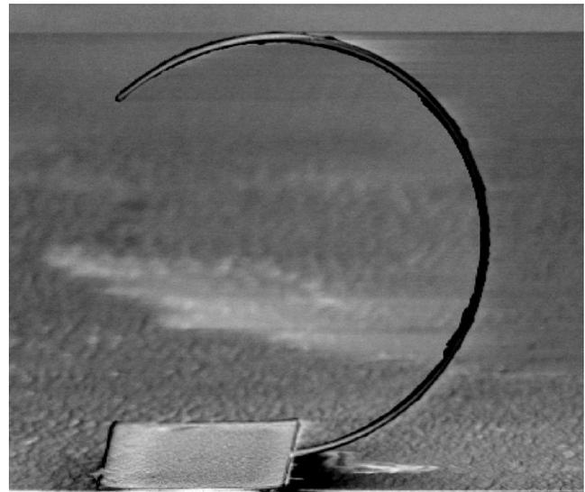
FIG. 2. Scanning electron micrograph of a loop composed of the AlN/GaN bilayer system created by the strain-induced self-rolling. The strip stretches in the AlN[11 $\bar{2}$ 0] direction. The width of the strip is 1  $\mu\text{m}$ . The radius of the loop is 11  $\mu\text{m}$ . The thicknesses of the AlN and GaN layers are, respectively, 45 and 120 nm, i.e., heterostructure 1.
