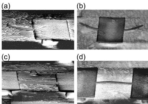
FIG. 1. Scanning electron micrograph of 200-nm-wide cantilevers, (a) and (b), and beams, (c) and (d). The cantilevers are 4.0  $\mu\text{m}$  long and the beams are 6.0  $\mu\text{m}$  long. The narrow strips of the AlN/GaN bilayer system extend in the [0001] direction in (a) and (c) and in the [11 $\bar{2}$ 0] direction in (b) and (d). The thicknesses of the AlN and GaN layers are, respectively, 45 and 120 nm, i.e., heterostructure 1.
