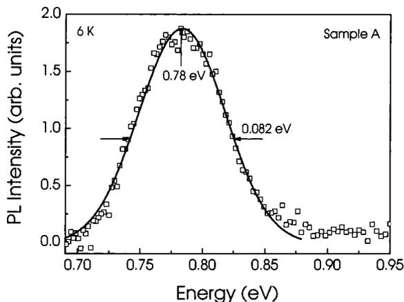
FIG. 4. PL spectrum at 6 K of sample A. The solid line is a Gaussian fit to the data for the determination of the FWHM and the peak energy position.
