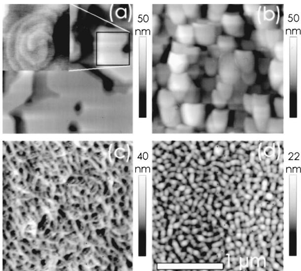
FIG. 1. AFM micrographs of InN layers (samples A–D) grown on a GaN buffer layer. The scale is indicated. The inset in (a) shows a  $0.5 \times 0.5 \mu\text{m}^2$  closeup of a plateau.
