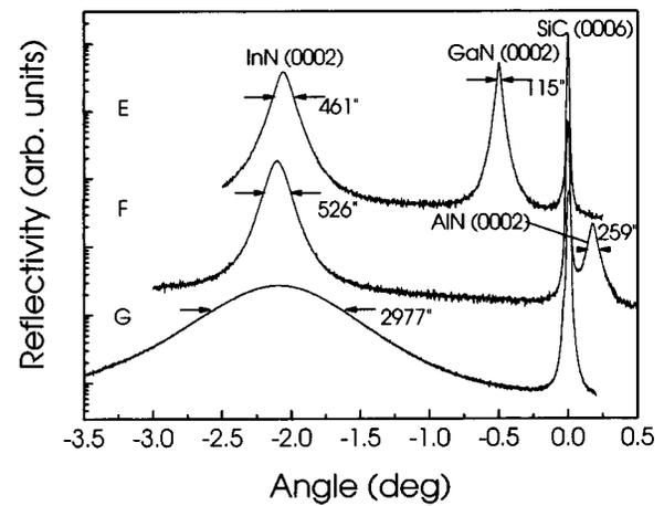
FIG. 2. X-ray rocking curves of InN layers grown at  $460^\circ\text{C}$  either on a GaN (sample E) or AlN (sample F) buffer or directly on the SiC substrate (sample G). The profiles are vertically offset for clarity.
