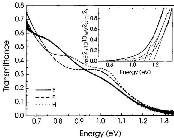
FIG. 3. Optical transmission spectra recorded at 300 K for three InN layers grown at 460 °C on GaN (samples E and H) or AlN (sample F) buffer layers. The fringes are due to thickness interferences. The inset shows the squared absorption coefficients vs. photon energy and linear extrapolations indicating the band gaps of the three samples.
