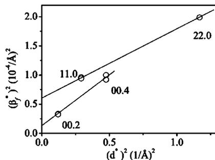
FIG. 7. Williamson-Hall plot in the reciprocal-lattice representation for the Gaussian line profiles.  $d^*$  is the reciprocal-lattice vector and  $\beta_f^* = \beta_f \cos(\Theta)/\lambda$ , where  $\beta_f$  is the integral breadth of the physically broadened profile.
