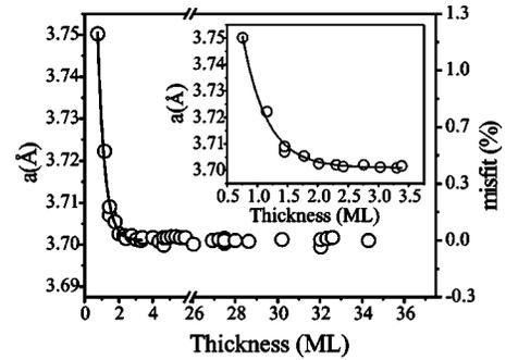
FIG. 6. Lattice parameter  $a$  as a function of the thickness of the growing layer. The line fitted to the data is an exponential decay function. The inset presents an enlarged plot of the initial phase of the growth. The MnAs films is already fully relaxed at a thickness of 2.5 monolayers (ML). The corresponding error bars are smaller than the symbols.
