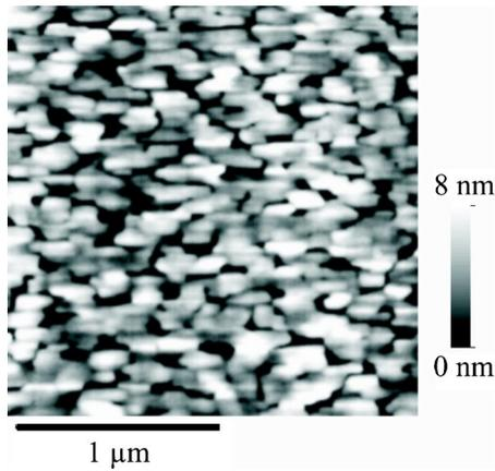
FIG. 1. Atomic force micrograph of the sample surface after the growth was finished, revealing an MnAs island pattern on the GaAs surface.
