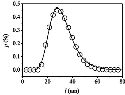
FIG. 9. Volume-weighted distribution function (circles) along MnAs [00.1]. The line is a fit by a lognormal function. This function demonstrates the possible fluctuations of the domain sizes.
