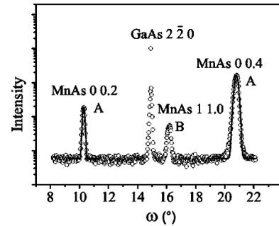
FIG. 3. X-ray grazing incidence diffraction curve ( $\omega/2\theta$  scan, circles) measured at a substrate temperature of 200 °C along the GaAs  $[1\bar{1}0]$  direction with the GaAs  $2\bar{2}0$  substrate and the MnAs 00.2 and 00.4 layer reflections (from the domains in A orientation). The MnAs 11.0 reflection from the domains in B orientation is also visible. The MnAs 00.2 and 00.4 peaks are fitted to the Gaussian functions (solid lines).
