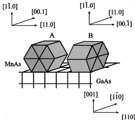
FIG. 2. Schematic view of the epitaxial relationship of MnAs on GaAs(001). The A and B orientations of the MnAs film are shown.
