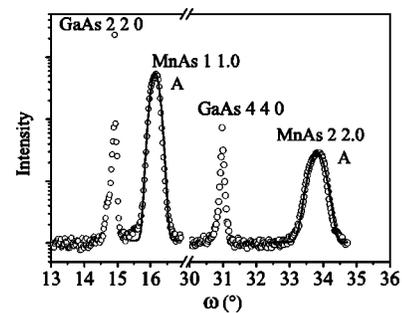
FIG. 4. X-ray grazing incidence diffraction curves ( $\omega/2\theta$  scans, circles) measured at a substrate temperature of 200 °C along GaAs  $[110]$  with the GaAs 220 and 440 substrates and the MnAs 11.0 and 22.0 layer reflections of the domains in A orientation. The MnAs 11.0 and 22.0 peaks are fitted to the Gaussian functions (solid lines).
