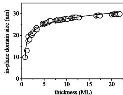
FIG. 8. Average in-plane domain size  $l$  vs the layer thickness measured in the monolayers (ML) during the growth. The size was calculated according to Eq. (4).
