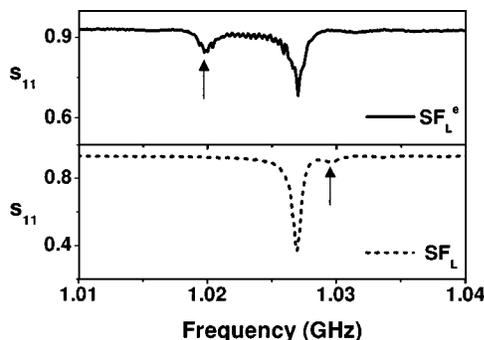
FIG. 6. rf reflection coefficient  $s_{11}$  of IDTs SF<sub>L</sub><sup>e</sup> (a) and SF<sub>L</sub> (b) determined using a network analyzer. The arrows indicate the first-order mode for each case.
