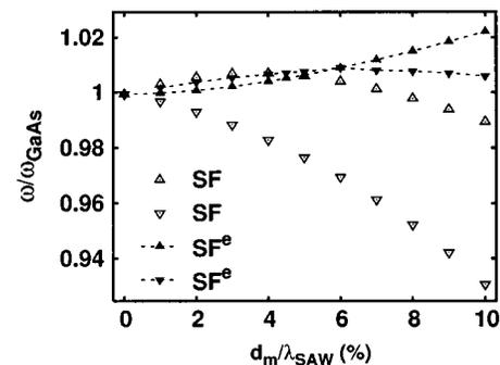
FIG. 3. Dependence of the frequency of the SAW modes  $\omega^+$  and  $\omega^-$  defining the stop band of SF IDT gratings on the thickness  $d_m$  of the Al metallization. The open and solid symbols correspond to normal and embedded gratings, respectively. The frequencies are normalized to that of the mode with wave vector  $\pi/\lambda_{\text{IDT}}$  on the bare GaAs substrate. The symmetry of the modes is described in the caption of Fig. 2.
