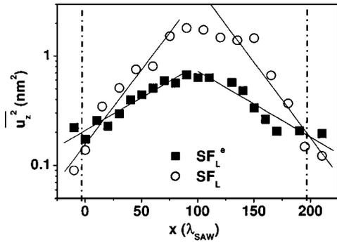
FIG. 7. Profiles of the squared vertical displacement  $\overline{u_z^2}$  along the IDT length ( $x$  direction) of the linear  $SF_L^e$  and  $SF_L$  IDTs determined by interferometry. The dot-dashed lines at  $x=0$  and  $200\lambda_{SAW}$  mark the edges of the IDTs.
