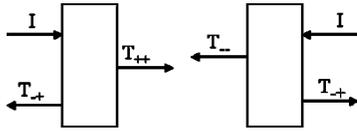
FIG. 3. Definitions of transmission and reflection coefficients.
