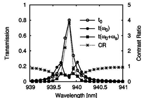
FIG. 5. Calculated transmission coefficient near  $\omega_0=940$  nm for the structure given in Fig. 2 with (solid symbols) and without a SAW (open symbols). The wavelength scale is in the vicinity of the cavity resonance displayed in Fig. 4. The dotted line shows the contrast ratio CR.
