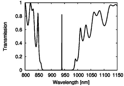
FIG. 4. Calculated transmission coefficient for the structure given in Fig. 1 in the absence of a SAW. The sharp line at 940 nm corresponds to the cavity resonance.
