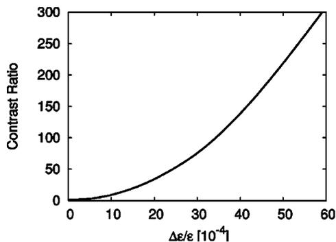
FIG. 6. Expected contrast ratio of the 1D optical switch as a function the dielectric modulation  $\eta = \Delta\epsilon/\epsilon$
