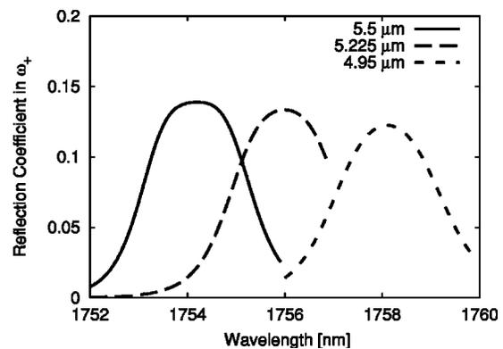
FIG. 11. Reflection coefficient for the up-shifted mode  $\omega_s$  of the structure of Fig. 8, calculated for three different SAW wavelengths.
