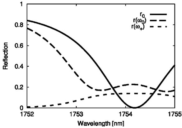
FIG. 9. Calculated reflection coefficient near the resonance wavelength of 1754 nm for the structure given in Fig. 8 in the absence of a SAW (solid line) and under a SAW with wavelength of 5.5  $\mu\text{m}$  for the unshifted [ $r(\omega_0)$ , dashed line] and for the up-shifted [ $r(\omega_0 + \omega_s)$ , dotted line] modes.
