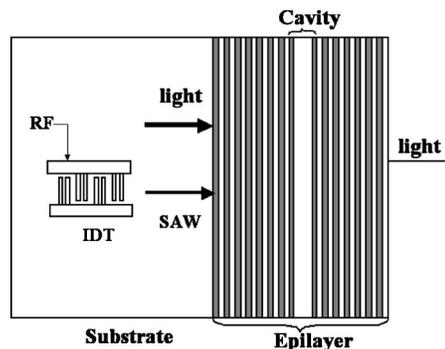
FIG. 7. One-dimensional cavity structure modulated by a SAW.
