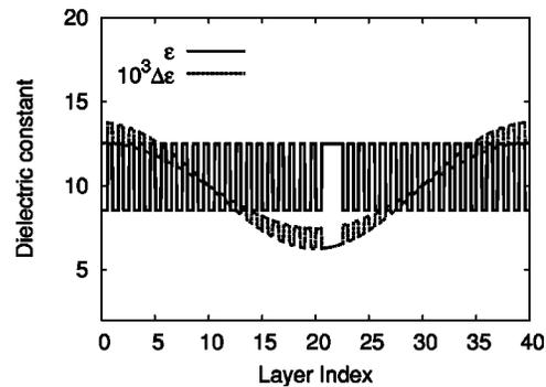
FIG. 2. Dielectric constant (solid line) and dielectric modulation by an acoustic wave (dashed line) in a one-dimension PBG structure consisting of a GaAs cavity inserted in-between asymmetric GaAs/AlAs Bragg mirrors.
