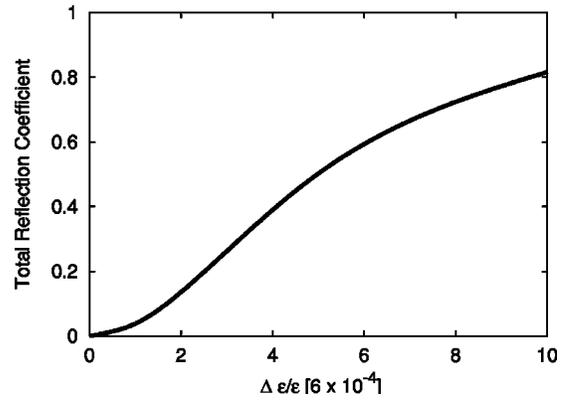
FIG. 10. Expected total reflection coefficient of the 2D structure of Fig. 8 as a function of  $\eta = \Delta\epsilon/\epsilon$ .
