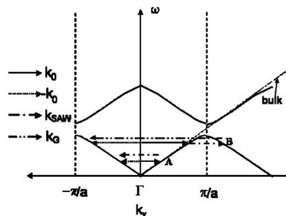
FIG. 1. Light dispersion in an unstructured (dashed line) and in a one-dimensional PBG structure. The arrows indicate a direct (a) and an umklapp (b) scattering process induced by a SAW with wave vector  $\mathbf{k}_{\text{SAW}}$ , which can be employed for frequency-tunable light filter.
