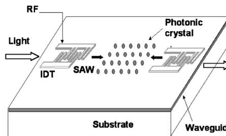
FIG. 8. Proposed two-dimensional PBG structure based on semiconductors.
