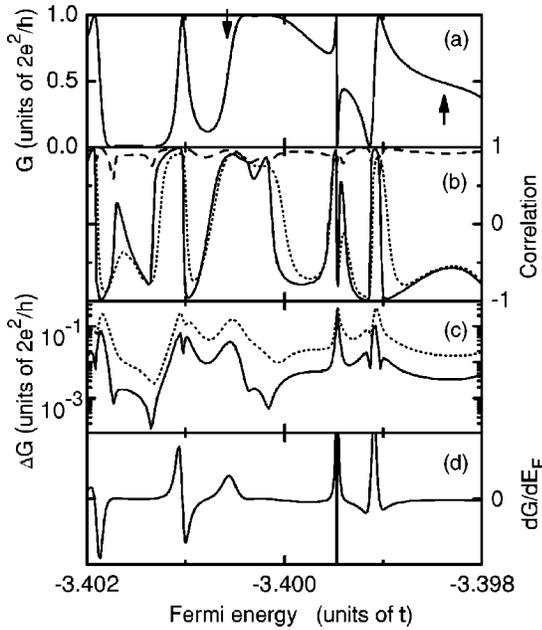
FIG. 3. (a) Magnetoconductance, (b) correlations  $C$  and  $\tilde{C}$  (dashed line), and (c) magnitude of conductance change  $\Delta G$  in a stadium cavity. The derivative  $dG/dE_F$  of the conductance curve is shown in (d). In (b) and (c),  $U=0.1t$  and  $0.5t$  for the solid and dotted lines, respectively. For  $\tilde{C}$  in (b),  $U=0.1t$ . The arrows in (a) indicate the energies at which the plots in Fig. 4 are calculated.
