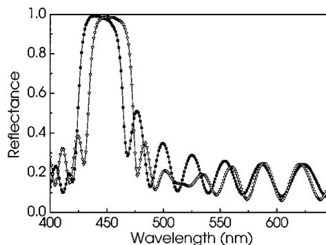
FIG. 2. Reflectance spectra of an undoped DBR (filled squares) and a doped DBR (open triangles).
