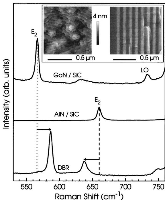
FIG. 1. Raman spectra of thick GaN (top) and AlN (center) films and an undoped DBR structure (bottom). The left picture in the inset shows an AFM micrograph of the surface of an undoped DBR taken over a  $1 \times 1 \mu\text{m}^2$  area. The right picture in the inset shows an SEM image of a cross section (sideview) of the undoped DBR in Fig. 1.
