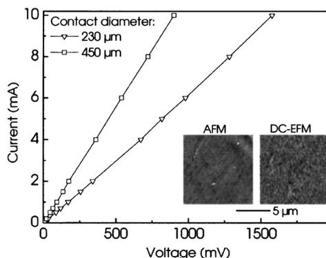
FIG. 3. Vertical  $I$ - $V$  measurements of a doped DBR done at room temperature using two different contact diameters. The right image in the inset shows a DC-EFM map of the surface of a doped DBR taken over a  $10 \times 10 \mu\text{m}^2$  area. The left image shows the corresponding AFM micrograph of the same area.
