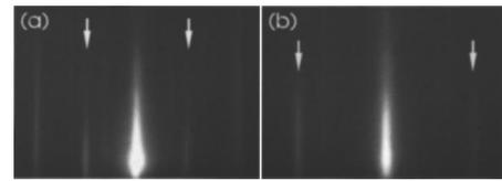
FIG. 3. RHEED patterns taken along the (a)  $\langle 11\bar{2}0\rangle$  and (b)  $\langle 1\bar{1}00\rangle$  azimuths of 6H-SiC at the end of the  $\text{Mn}_4\text{N}$  deposition for a sample grown at very high Mn/N flux ratio.
