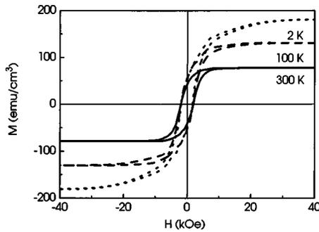
FIG. 4. Magnetization loop obtained at different temperatures. The magnetic field is applied perpendicular to the sample surface; that is, parallel to the  $c$  axis.
