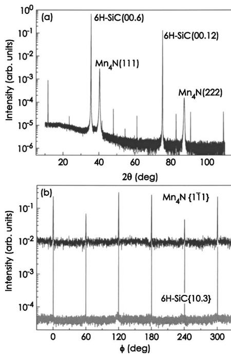
FIG. 2. (a) Symmetric x-ray  $\omega/2\theta$  scan of a  $\text{Mn}_4\text{N}$  film grown on 6H-SiC(0001). (b)  $\phi$  scans of the  $\{10.3\}$ -planes of 6H-SiC and the  $\{1\bar{1}1\}$ -planes of  $\text{Mn}_4\text{N}$ . The peaks, not labeled in (a) are due to forbidden reflections of 6H-SiC.
