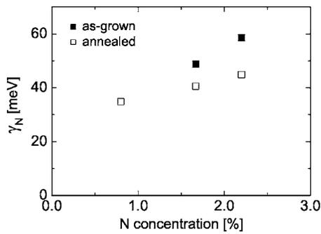
FIG. 3. Mean square N induced potential fluctuation  $\gamma_N$  as a function of the N concentration.
