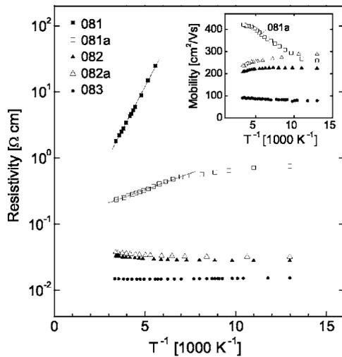
FIG. 1. Temperature dependence of the resistivity for samples containing 0.8% N with different electron concentrations. The inset shows the mobility for the corresponding samples. The solid lines are least-square linear fits of the data.
