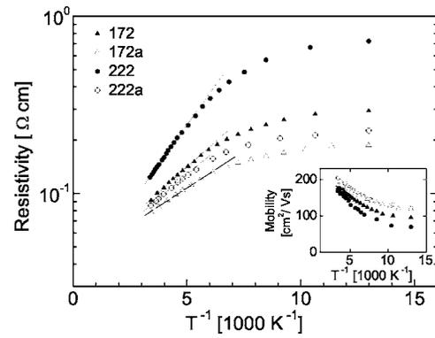
FIG. 2. Temperature dependence of the resistivity for samples containing 1.7% and 2.2% N. The inset shows the mobility for the corresponding samples. The solid lines are least-square linear fits of the data.
