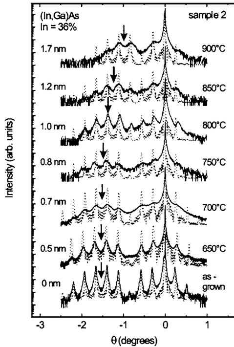
FIG. 2. XRD curves around the (004) reflection of the (In,Ga)As sample with 36% indium (sample 2) annealed at different temperatures for 60 s. The arrows denote the envelope maxima. The dotted lines refer to the computer simulation. The left-hand side number represents the diffusion lengths  $x_D$  employed for the simulations.
