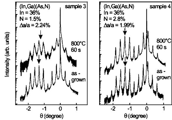
FIG. 3. XRD curves around the (004) reflection of the (In,Ga)(As,N) samples comprising 36% indium as well as 1.5% and 2.8% nitrogen (samples 3 and 4). The maxima of the envelope are denoted by the arrows.
