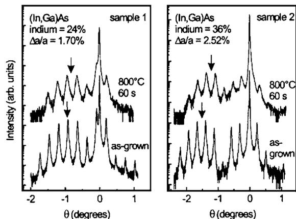
FIG. 1. XRD curves around the (004) reflection of the  $(\text{In,Ga})\text{As}$  samples comprising 24% and 36% indium (samples 1 and 2). The maxima of the envelope are denoted by the arrows.
