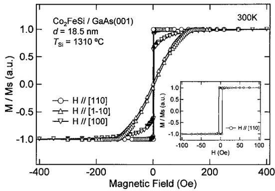
FIG. 4. Magnetization curves for 18.5 nm thick stoichiometric  $\text{Co}_2\text{FeSi}/\text{GaAs}(001)$  film grown at  $100^\circ\text{C}$ . The inset shows an expanded view of the magnetization curve along the  $[110]$  direction. After subtraction of the diamagnetic contribution of the GaAs substrate, the magnetizations were normalized to the saturation magnetization in each direction.
