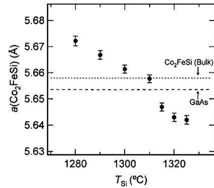
FIG. 2. Dependence of the unstrained lattice constant of  $\text{Co}_2\text{FeSi}$  layers ( $a_{\text{Co}_2\text{FeSi}}$ ) on Si cell temperature. The broken line and the dashed line indicate the bulk value of  $\text{Co}_2\text{FeSi}$  and GaAs, respectively.
