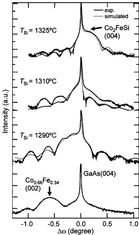
FIG. 1. Normalized  $\omega$ - $2\theta$  curves for  $\text{Co}_2\text{FeSi}/\text{GaAs}(001)$  and  $\text{Co}_{0.66}\text{Fe}_{0.34}/\text{GaAs}(001)$  (bottom line) films grown at  $100^\circ\text{C}$  with various Si cell temperatures together with the simulated curve using the Takagi-Taupin formalism (dotted lines).
