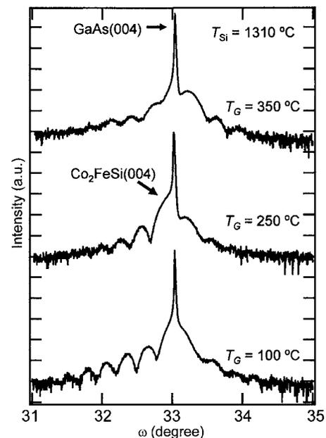
FIG. 3. Normalized  $\omega$ - $2\theta$  curves for stoichiometric  $\text{Co}_2\text{FeSi}/\text{GaAs}(001)$  films grown at various growth temperature ranging from  $100^\circ\text{C}$  to  $350^\circ\text{C}$ .
