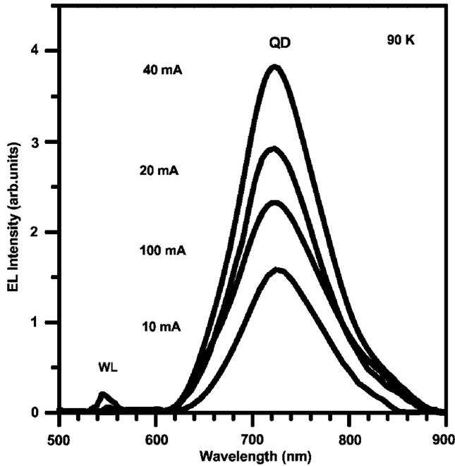
FIG. 1. Current dependence of the EL spectra at 90 K.
