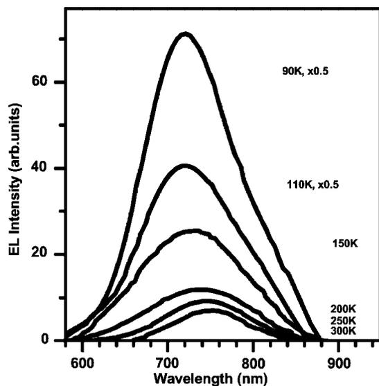
FIG. 3. Temperature evolution of the EL spectra under constant current of 100 mA.
