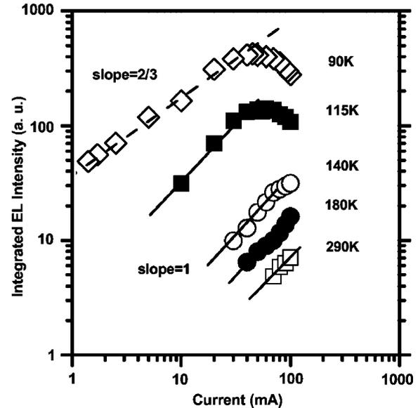
FIG. 2. Current dependence of the integrated EL intensity for several temperatures. The dashed and solid lines show slopes of 2/3 and 1, respectively.
