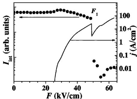
FIG. 4. Integrated PL intensity  $I_{\text{int}}$  of the interband PL transition lowest in energy and current density  $j$  as a function of  $F$  for the GaAs/Al<sub>0.45</sub>Ga<sub>0.55</sub>As QCS. At  $F_1$ , an abrupt decrease of the PL intensity is observed.
