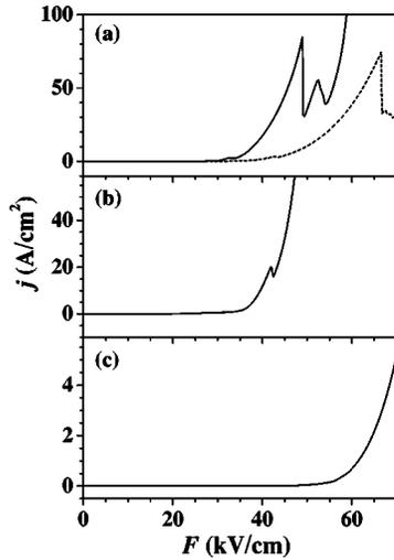
FIG. 1.  $I$ - $V$  characteristics (a) of the GaAs/Al<sub>0.33</sub>Ga<sub>0.67</sub>As QCS with Ohmic (solid line) as well as Schottky (dashed line) contacts, (b) of the GaAs/Al<sub>0.33</sub>Ga<sub>0.67</sub>As QCS with the modified first period, and (c) of the double-quantum-well superlattice.
