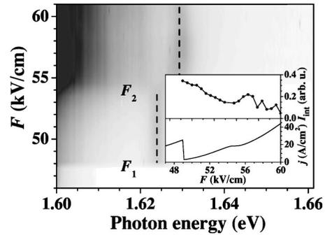
FIG. 5. Normalized PL spectrum in the vicinity of the lower laser level for the GaAs/Al<sub>0.45</sub>Ga<sub>0.55</sub>As QCS as a function of  $F$  in a gray-scale representation. The inset shows the dependence of  $I_{\text{int}}$  of the PL line from the lower laser level and  $j$  on  $F$ . The vertical dashed lines indicate the different PL peak positions of the lower laser level for  $F < F_2$  and  $F > F_2$ .
