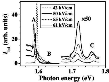
FIG. 6. PL spectra of the GaAs/Al<sub>0.45</sub>Ga<sub>0.55</sub>As QCS recorded for different electric field strengths as indicated showing the ground-state transition (A), the lower laser level (B), and the upper laser level (C). The PL spectra at higher energies (1.67–1.78 eV) have been multiplied by a factor of 50 and shifted vertically for clarity.
