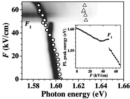
FIG. 3. Normalized, electric-field-dependent PL spectra of the conduction-band ground state and the lower laser level of the GaAs/Al<sub>0.45</sub>Ga<sub>0.55</sub>As QCS in a gray-scale representation. For comparison, the calculated transition energies for the ground state (circles) and lower laser level (triangles) are added. The inset shows the dependence of the peak energy of the ground state on the electric field strength  $F$ .
