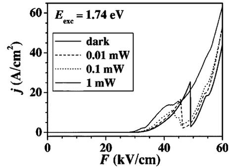
FIG. 7.  $I$ – $V$  characteristics under illumination for different excitation powers at an excitation energy of 1.74 eV for the GaAs/Al<sub>0.45</sub>Ga<sub>0.55</sub>As QCS.
