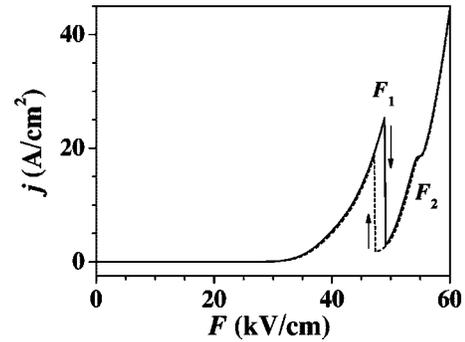
FIG. 2.  $I$ - $V$  characteristics of the GaAs/Al<sub>0.45</sub>Ga<sub>0.55</sub>As QCS for an up sweep (solid line) and a down sweep (dashed line).  $F_1$  and  $F_2$  denote the field strengths for NDC.
