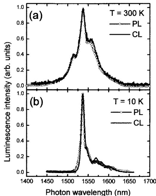
FIG. 7. Photo- (PL) and cathodoluminescence (CL) spectra of an Er-doped *a*-AlN film annealed at 900 °C. The spectra have been achieved at room temperature (a) and at 10 K (b) by means of 488.0 nm photons (PL) or 10 keV electrons (CL). The main feature at 1532 nm corresponds to the  ${}^4I_{13/2} \rightarrow {}^4I_{15/2}$  optical transition due to Er<sup>3+</sup> ions. The spectra have been normalized for comparison purposes.
