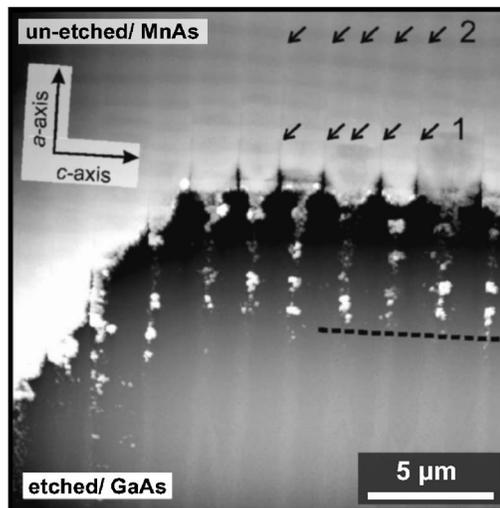
FIG. 5. AFM image at the border between the etched and unetched areas of a 215-nm-thick MnAs film. The film was etched at room temperature, i.e., in the  $\alpha$ - $\beta$ -stripe phase, again showing a large underetching. The unetched parts of the film show the coexisting phases oriented along the  $c$  axis and, perpendicular to them, regularly spaced bright stripes (see arrows labeled '2') that originate from cracks at the etch front (see arrows labeled '1').
