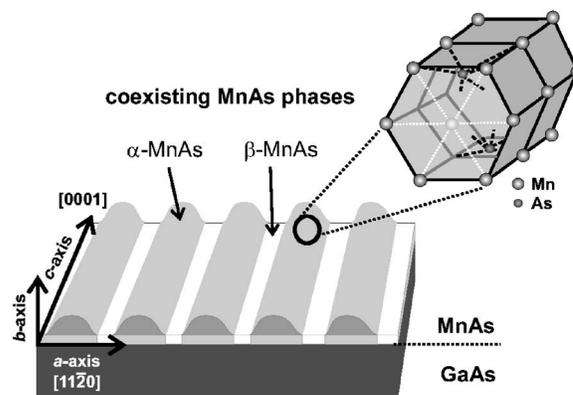
FIG. 1. Sketch of the stripe structure of the strain-stabilized coexisting  $\alpha$ - and  $\beta$ -MnAs phases on GaAs(001) in the temperature range from 10 to 40 °C. The in-plane  $a$  axis is the easy axis of magnetization and the magnetic hard axis is along the in-plane  $c$ -axis direction (MnAs[0001]). On the top right, a detailed sketch of the hexagonal  $\alpha$ -MnAs cell is shown.
