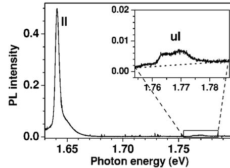
FIG. 1. PL spectrum of sample A1 ( $x=0.33$ ) at 56 kV/cm. The inset depicts a magnification for the energy range of the upper laser level. The dotted line in the inset indicates the assumed background signal.
