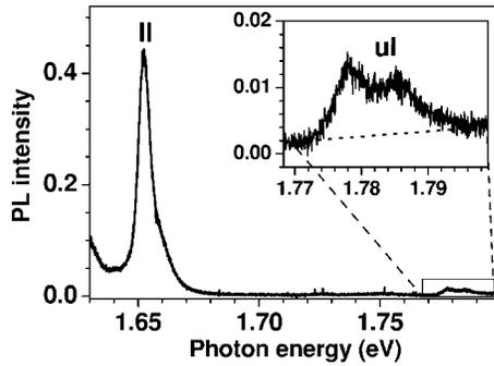
FIG. 2. PL spectrum of sample A2 ( $x=0.33$ ) at 56 kV/cm. The inset depicts a magnification for the energy range of the upper laser level. The dotted line in the inset indicates the assumed background signal.
