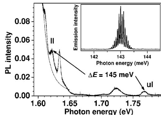
FIG. 4. Magnified part of the high-energy region of the PL spectrum shown in Fig. 3. The dotted line indicates a Lorentzian fit to the two peaks with the lowest energy used for the estimation of the background intensity. The inset presents a laser spectrum for one of the corresponding QCLs.
