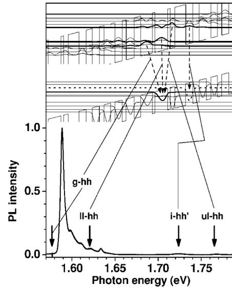
FIG. 3. PL spectrum of sample B ( $x=0.45$ ) at 60 kV/cm. The top part shows a schematic view of the subband structure and the possible interband transitions.
