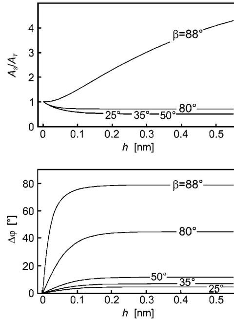
FIG. 5. Relative amplitude  $A_S/A_T$  and phase-shift  $\Delta\varphi$  as a function of the step height  $h$  with the STM tip being 1-nm above the step edge and  $\kappa = 10 \text{ nm}^{-1}$ ;  $A_T$  and  $A_S$  are the amplitude of the mixing signal at the terrace and step, respectively.
