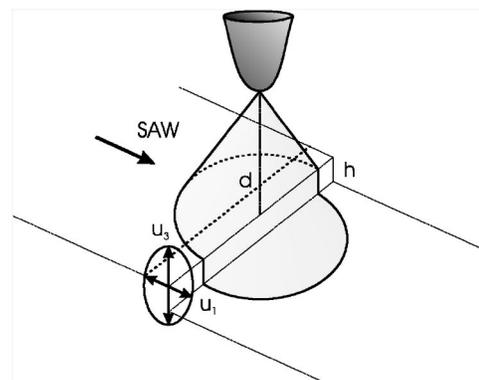
FIG. 4. Schematic illustration of the tunneling current arising at an oscillating step while being scanned by the STM tip at a distance  $d$ : The step of height  $h$  separates two extended flat terraces and runs perpendicular to the propagation direction of the SAW. The entire surface, including the step, oscillates with the frequency  $\omega$  of the SAW, with each point following a trajectory defined by the longitudinal ( $u_1$ ) and vertical ( $u_3$ ) SAW amplitudes.
