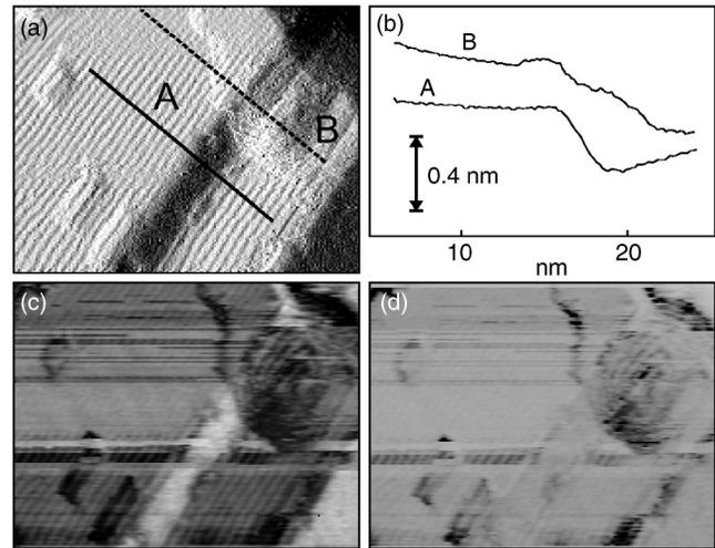
FIG. 7. (a)  $34 \times 25$  nm<sup>2</sup> differentiated STM image (left) of a 100-m-thick Au film on Y-cut LiNbO<sub>3</sub> as well as of two linescans of steps (right) marked by A and B in the topview. (b) Corresponding amplitude and (c) phase image of a Rayleigh wave, both recorded simultaneously with topography. Note the strong enhancement of the amplitude contrast at the steep step (linescan A).
