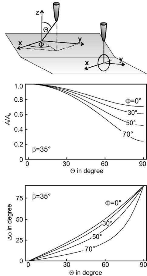
FIG. 3. Relative amplitude  $A/A_h$  and phase-shift  $\Delta\varphi$  as a function of the inclination angle  $\Theta$  for different azimuthal tilts  $\Phi$  calculated by Eqs. (1) and (2), respectively; polar and azimuthal angles  $\Theta$  and  $\Phi$  are illustrated in the sketch;  $A$  and  $A_h$  are the amplitude of the mixing signal at the horizontal and inclined plane, respectively.
