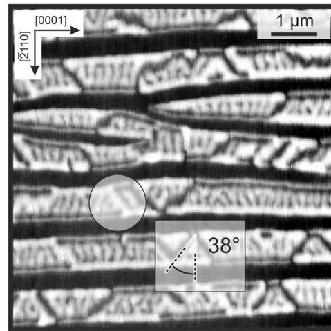
FIG. 3. MFM image of a 215-nm-thick MnAs layer on GaAs(001) in the  $\alpha+\beta$  phase coexistence region at 293 K. The scan size is  $7 \times 7 \mu\text{m}^2$ .
