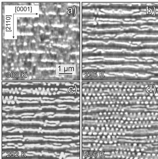
FIG. 2. MFM images of a 180-nm-thick MnAs layer on GaAs(001) in the  $\alpha+\beta$  phase coexistence region at different temperatures. The scan size is  $7 \times 7 \mu\text{m}^2$ .
