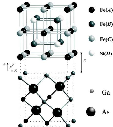
FIG. 1. (Color online) Schematic view of the D0<sub>3</sub> unit cell of Fe<sub>3</sub>Si grown epitaxially on GaAs. The A and C sites are equivalent and are occupied by Fe. The B sites are also occupied by Fe, whereas the D sites are occupied by Si. In the epitaxial system, the first layer of Fe atoms is located at the positions of the Ga atoms in the GaAs lattice. The vertical shift  $z$  is enlarged for clarity. The choice of the radii of the atoms is arbitrary.
