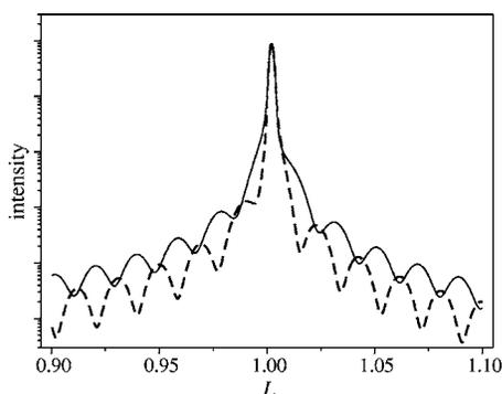
FIG. 2. Calculated CTRs at the 111 reflection from a stoichiometric fully ordered Fe<sub>3</sub>Si layer (30 nm thick) on GaAs(001) for the lattice registry shown in Fig. 1 (full line) and for the case of the Fe<sub>3</sub>Si structure shifted by 1/2 of the unit cell in the (100) direction (broken line).
