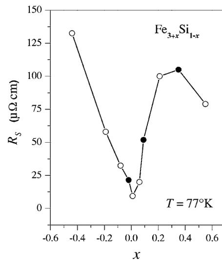
FIG. 6. Resistivity  $R_S$  of several  $\text{Fe}_3\text{Si}$  films measured at 77 K as a function of the deviation  $x$  from stoichiometric composition. The three samples investigated by grazing incidence diffraction are marked by full circles.
