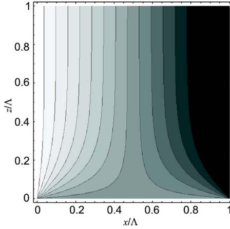
FIG. 6. (Color online) Contour plot of the displacement field due to the periodic dislocations at the interface. Distribution in the plane normal to the surface and normal to the dislocation lines according to Eq. (3). The contour lines are almost parallel to each other for a thickness larger than  $\Lambda/\pi$ .
