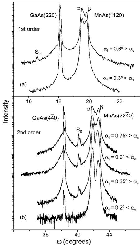
FIG. 7. Radial ( $\omega/2\theta$ ) scans recorded along the  $a$  axis of the MnAs/GaAs(113)A interface for different grazing incidence angles  $\alpha_i$ . (a) First- and (b) Second-order reflection. The  $S_i$  indicate the satellites originating from the periodic array of misfit dislocations. The scans are recorded at room temperature. Peaks labelled  $\alpha$  and  $\beta$  refer to the different phases of MnAs. The profiles are shifted vertically for clarity. X-ray energy, 10 keV.
