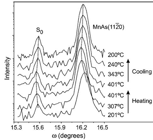
FIG. 8. Radial ( $\omega-2\theta$ ) scans along the MnAs[11 $\bar{2}0$ ] direction measured in GID geometry during *in situ* post-growth annealing. The scans were recorded at a grazing incidence angle of 0.3°. The temperature is given to the right of each curve. For clarity, the curves are shifted in the vertical direction. The dotted lines on the curves are guides to the eye for the peak position at different temperatures. X-ray energy, 12 keV.
