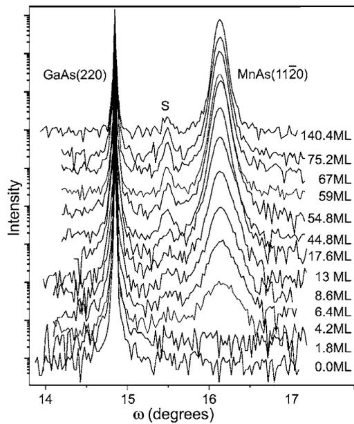
FIG. 2. X-ray diffraction curves ( $\omega/2\theta$  scans) measured *in situ* during growth at 250 °C along the GaAs[110] direction. The scan includes the GaAs(220) substrate and the MnAs(11 $\bar{2}$ 0) layer reflections. The scans are recorded at a grazing incidence angle of 0.2°. The deposited number of monolayers is indicated to the right of each scan. The curves are shifted vertically for clarity. X-ray energy, 12 keV.
