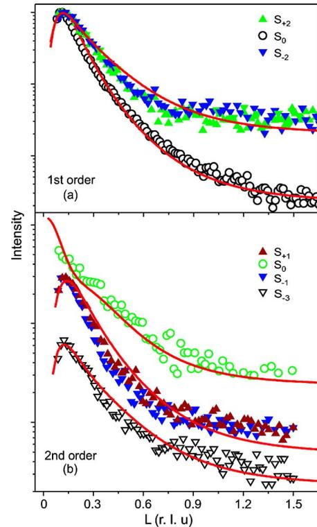
FIG. 5. (Color online) Intensity variation along the crystal truncation rods of different observed satellites originating at the first- and second-order reflection, shown in Figs. 4(a) and 4(b). The continuous (red) lines show the calculated CTRs of the different satellites. No fit parameters are used to match the calculated CTRs with the measured intensity profiles. The profile in (b) is shifted vertically for clarity. X-ray energy, 10 keV.
