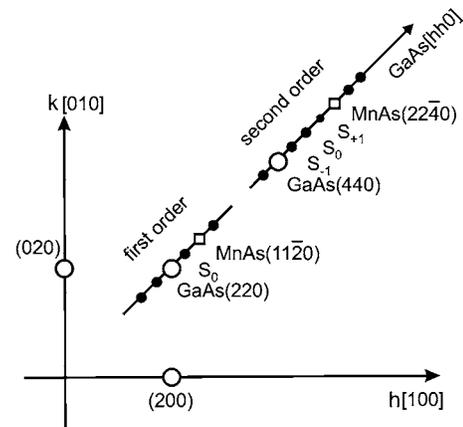
FIG. 1. Schematic representation of the  $(hk0)$  reciprocal space plane of MnAs/GaAs(001) with an array of misfit dislocations at the interface. The large open circles and the squares correspond to the GaAs and MnAs Bragg peaks, respectively. The filled circles represent the position of observed satellite reflections from the dislocation array along GaAs[110]. Two orders of scans with all observed reflections are included.
