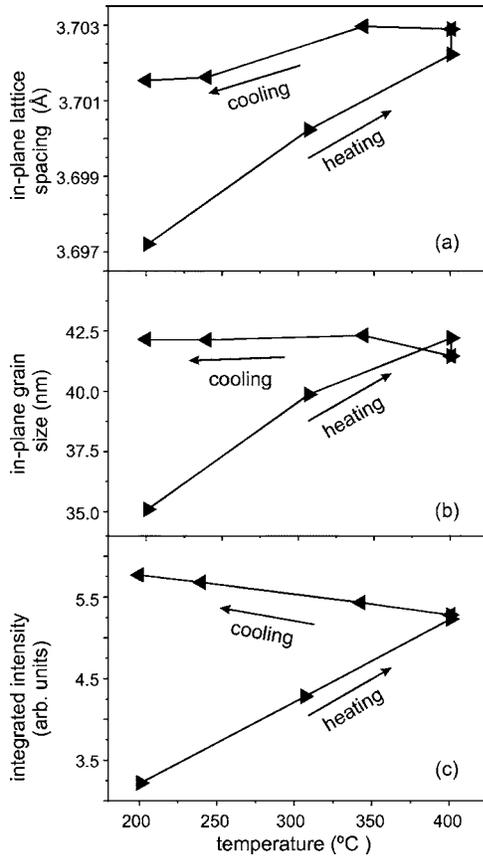
FIG. 9. The evolution of in-plane lattice spacing (a), in-plane grain size (b), and integrated intensity (c) along the  $a$  axis during *in situ* post-growth thermal annealing as a function of annealing temperature. The arrows indicate the direction of heating to 400 °C and subsequent cooling to 200 °C. The filled triangles pointing right represent the measurement during heating. The triangles pointing left represent the measurement during cooling.
