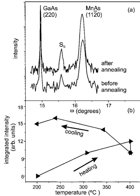
FIG. 10. (a) Radial ( $\omega/2\theta$ ) scans along the MnAs[11 $\bar{2}$ 0] direction measured at 200 °C before and after annealing. (b) The evolution of integrated intensity of the  $S_0$  satellite during annealing. The intensity increases 2.5 times during annealing. Arrows indicate the heating and cooling sequence. X-ray energy, 12 keV.
