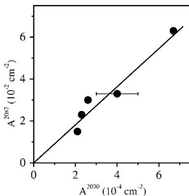
FIG. 4. Correlation between the integrated intensities  $A$  of the absorption lines at  $2087.12\text{ cm}^{-1}$  and  $2030.66\text{ cm}^{-1}$ . The straight line corresponds to the  $[^{13}\text{C}]/[^{12}\text{C}]=0.011$  ratio of the carbon natural abundances.
