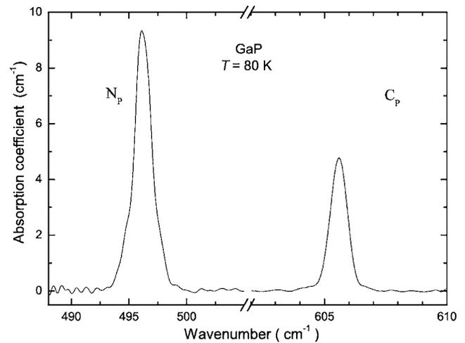
FIG. 3. Spectra of the local vibrational modes of substitutional nitrogen and substitutional carbon measured at  $T=80$  K on a GaP sample; in that sample,  $[N_p]=1.5 \times 10^{17}$   $\text{cm}^{-3}$  and  $[C_p]=3.7 \times 10^{16}$   $\text{cm}^{-3}$ . The background due to the two-phonon absorption has been subtracted. The integrated intensity of the C—N stretching mode measured on this sample is  $A^{2087}=2.3 \times 10^{-2}$   $\text{cm}^{-2}$  (cf. Fig. 4).
