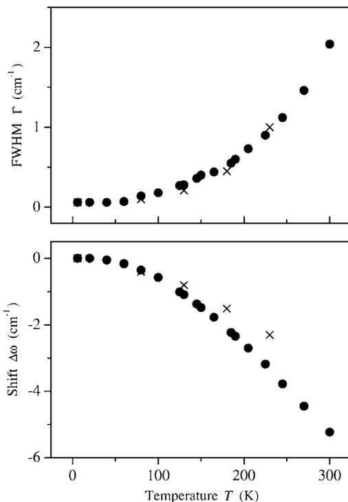
FIG. 2. Temperature dependence of the shift  $\Delta\omega$  of the line position and FWHM  $\Gamma$  of the  $2087.12$   $\text{cm}^{-1}$  line (circles). The crosses are the data points for the  $2088.50$   $\text{cm}^{-1}$  line in GaAs.
