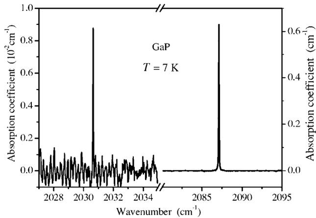
FIG. 1. Absorption spectrum of GaP measured at  $T=7$  K with an unapodized resolution of  $0.04$   $\text{cm}^{-1}$ . The line at  $2087.12$   $\text{cm}^{-1}$  is due to the  $^{12}\text{C}-^{14}\text{N}$  stretching mode, the line at  $2030.66$   $\text{cm}^{-1}$  is due to the isotopically shifted  $^{13}\text{C}-^{14}\text{N}$  mode.
