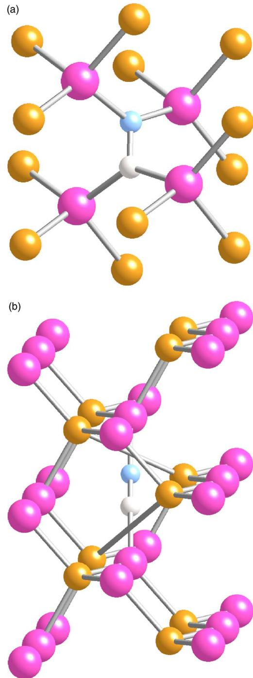
FIG. 7. (Color online) Ball and stick schematic representation of (a) a C—N radical substituting a phosphorus atom and (b) a C—N radical in a  $T_p$  interstitial site. The largest balls are gallium atoms, the intermediate size ones phosphorus atoms, and the two small balls the carbon and nitrogen atoms. The relaxation of the host atoms has not been represented.
