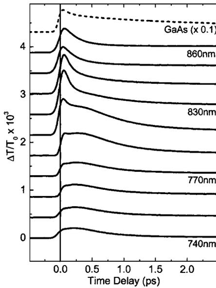
FIG. 1. Time resolved transmission changes of  $\text{GaN}_{0.013}\text{As}_{0.987}$  for different excitation wavelengths (from bottom: 740, 750, 760, 770, 790, 810, 830, 840, 850, and 860 nm, respectively) and of GaAs (dashed line, excitation wavelength 860 nm, scaled by 0.1). The curves are shifted vertically for clarity. The vertical line marks the zero time delay.
