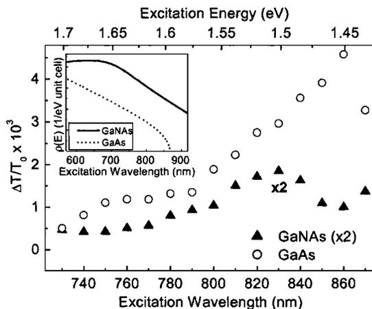
FIG. 2. Maximum of  $\Delta T/T_0$  around zero time delay of GaAs (open circles) and  $\text{GaN}_x\text{As}_{1-x}$  (filled triangles, scaled by a factor of 2) as function of the excitation wavelength. The inset shows the conduction band density of states of GaAs (dotted line) of  $\text{GaN}_{0.013}\text{As}_{0.987}$  (solid line).
