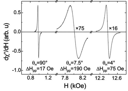
FIG. 2. FMR spectra of the stoichiometric sample A, taken at 9 GHz for three different polar orientations of the external magnetic field with  $\varphi_H=45^\circ$ .
