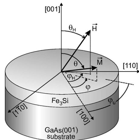
FIG. 1. Sketch of the coordinate system used.  $\varphi$  and  $\varphi_H$  are the azimuthal, and  $\theta$  and  $\theta_H$  are the polar angles of the magnetization  $\vec{M}$  and the external field  $\vec{H}$ , respectively.  $\varphi_u$  is the rotation of the easy axis of the uniaxial in-plane anisotropy with respect to the easy axis of the fourfold anisotropy.
