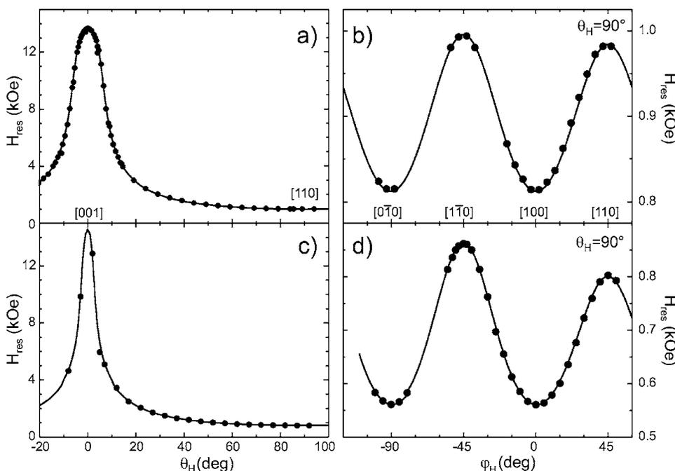
FIG. 4. (a) Polar and (b) azimuthal angular dependence of the resonance field measured at 9 GHz and ambient temperature, for the stoichiometric sample; (c) and (d) for the Fe-rich sample, respectively. The solid lines are fits according to Eqs. (3) and (4). The crystallographic directions are given in square brackets.
