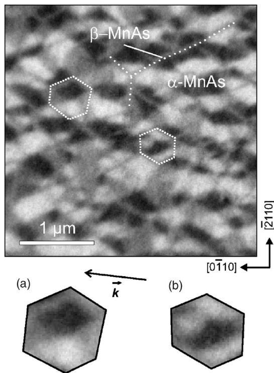
FIG. 2. Micromagnetic XMCDPEEM image of a 270-nm-thick MnAs film on GaAs(111)B recorded at 19 °C. The wave vector  $\mathbf{k}$  of the incident light is indicated below. Ferromagnetic  $\alpha$ -MnAs arranges in a network of quasi-hexagonal structures, separated by nonmagnetic  $\beta$ -MnAs. Two closeups of quasi-hexagonal elements reveal the common magnetization patterns: (a) vortex-like domain and (b) distorted stripe domain.
