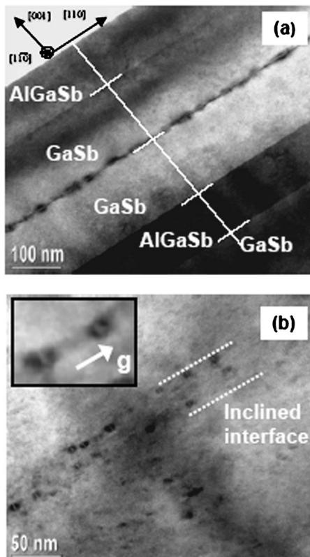
FIG. 2. TEM cross sectional images of 3 ML InSb QDs grown with the two step technique. Cross-sectional 002 bright-field (a) TEM of buried InSb QDs and projectional view (b) of tilted QDs layer ( $g=220$ ) in bright-field mode to visualize the isolated QDs. The inset in (b) is a zoom on two InSb QDs showing the characteristic coffee beam contrast of fully strained nanostructures.
