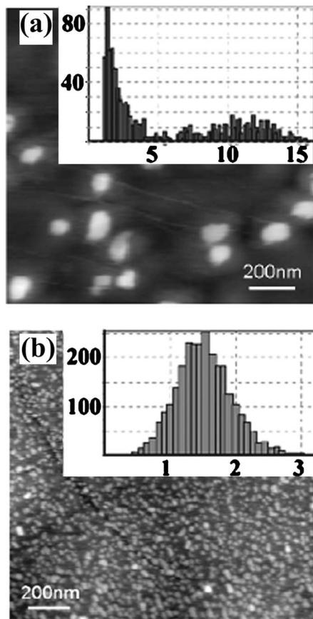
FIG. 1. AFM scan (size  $1 \times 1 \mu\text{m}^2$ ) on 2.6 ML of InSb deposited by the usual growth at  $450^\circ\text{C}$  (a) and deposited following the two step procedure (b). The insets are the related histograms for the height expressed in nm.
