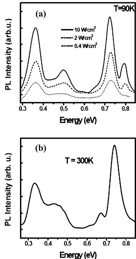
FIG. 3. PL spectra taken from the high density InSb/GaSb QD sample at 90 K (a) under different excitation intensities and at room temperature (b).
