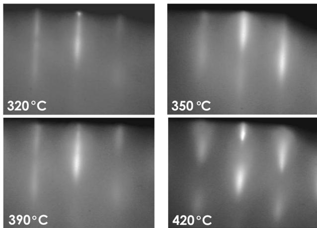
FIG. 1. RHEED patterns along the  $[1\bar{1}0]$  direction during the growth of 3 nm  $\text{Ga}_{0.6}\text{In}_{0.4}\text{N}_{0.04}\text{As}_{0.96}$  for the respective temperatures at a V/III BEP ratio of 5.
