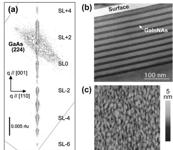
FIG. 3. Structural and morphological characteristics of the ten-period  $[(\text{Ga},\text{In})(\text{N},\text{As})$  (8 nm)/ $\text{Ga}(\text{N},\text{As})$  (14 nm)] MQW. (a) XRD reciprocal space map around the asymmetric  $\text{GaAs}(224)$  reflection, (b) cross-sectional TEM micrograph, and (c) AFM surface micrograph taken over an area of  $10 \times 10 \mu\text{m}^2$ . The root mean square roughness of this sample is 0.5 nm.
