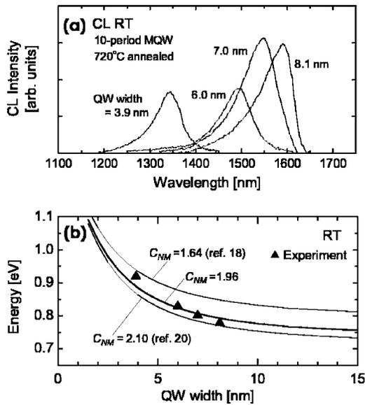
FIG. 4. (a) CL spectra for the ten-period  $\text{Ga}_{0.64}\text{In}_{0.36}\text{N}_{0.045}\text{As}_{0.955}/\text{GaN}_{0.008}\text{As}_{0.992}$  MQWs having different QW widths. The QW width obtained from the XRD fit is given for each spectrum. (b) Experimental and calculated CL peak energies vs QW width.
