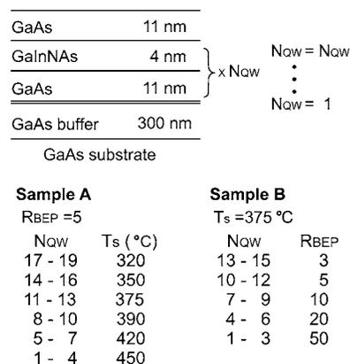
FIG. 1. Schemes of sample A and sample B.  $N_{\text{QW}}$  denotes the numbers of QWs. The growth conditions for each series of QWs are mentioned.
