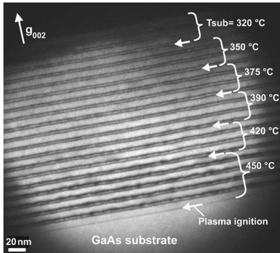
FIG. 2. Cross-sectional dark-field TEM micrograph ( $g=002$ ) of sample A. Growth interruptions before the growth of the first QW of each series are indicated by arrows.
