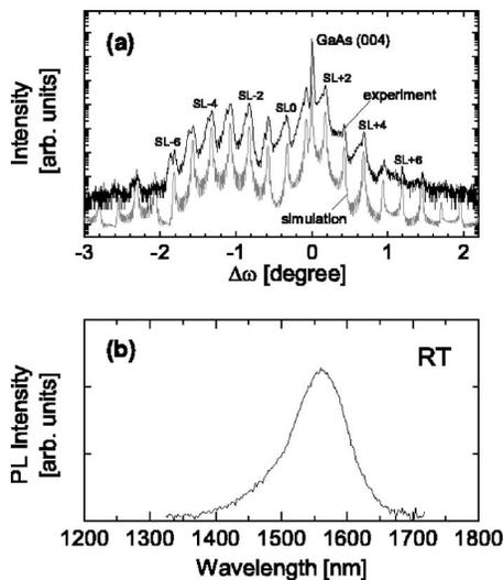
FIG. 4. (a) XRD  $\omega$ - $2\theta$  scans and (b) RT PL spectra for the ten-period (Ga,In)(N,As)/Ga(N,As) MQWs, showing emission at  $1.56 \mu\text{m}$ .
