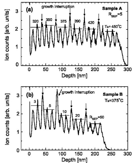
FIG. 3. SIMS depth profiles of N for (a) sample A and (b) sample B. The interfaces at which the growth interruptions were carried out are indicated by arrows. Varied parameters,  $T_s$  or  $R_{\text{BEP}}$ , are mentioned for each series of QWs. The parallel bars represent the averaged peak heights of the corresponding QWs for each series.
