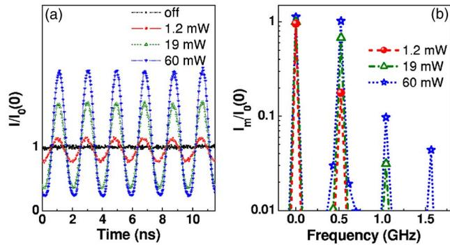
FIG. 2. (Color online) (a) Measured time-resolved light transmission ( $I$ ) through the MZI for different acoustic powers ( $P_{\text{IDT}}$ ), normalized to the value transmitted in the absence of a SAW [ $I_0(0)$ ]. (b) Fourier transformation (with components  $I_m$ ) of the transmitted intensity of the data displayed on (a).
