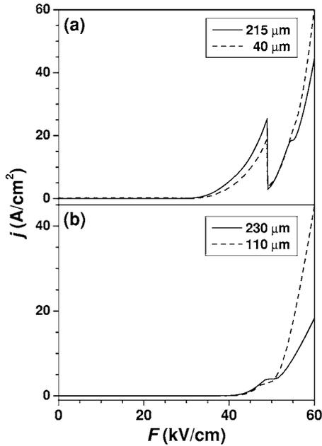
FIG. 3. Measured  $j$ - $F$  characteristics of (a) sample A for mesa diameters of 215  $\mu\text{m}$  (solid line) and 40  $\mu\text{m}$  (dashed line) as well as (b) sample B for mesa diameters of 230  $\mu\text{m}$  (solid line) and 110  $\mu\text{m}$  (dashed line) at 6 K. The field strength  $F$  was determined from the applied voltage divided by the thickness of 950 nm for sample A and 95 nm for sample B neglecting the contact layers.
