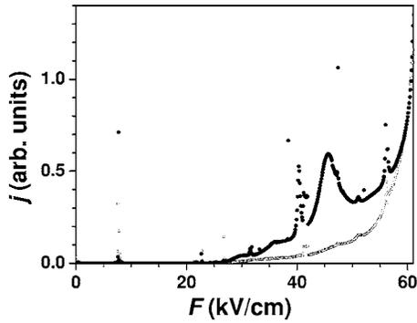
FIG. 2. Calculated  $j$ - $F$  characteristics for the structure of sample A neglecting field inhomogeneities without (circles) and with taking into account LO-phonon scattering (dots). The current density calculated without LO-phonon scattering has been multiplied by a factor of 12.
