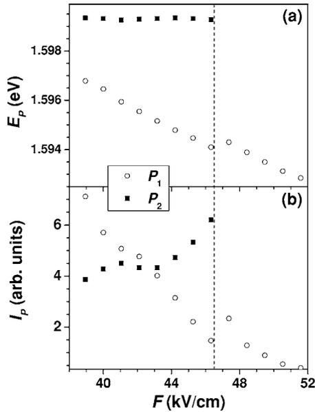
FIG. 5. (a) PL peak energies  $E_p$  and (b) integrated PL intensities  $I_p$  of the lower-energy peak  $P_1$  (circles) and the higher-energy peak  $P_2$  (squares) of the spectra shown in Fig. 4(b) as a function of electric field  $F$ . The energies and integrated intensities were obtained by fitting the spectra to two Lorentzians. The vertical dashed line indicates the critical field strength  $F_{crit}$ , where bistable behavior is observed.
