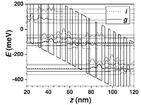
FIG. 1. Calculated conduction band profile, energy levels, and electron probability density at  $F=45.5$  kV/cm for the structure of sample A neglecting field inhomogeneities. The ground state  $g$  in the active region and the intermediate injector state  $i$  are marked by the thick solid and dotted lines, respectively.
