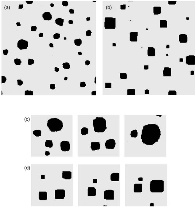
FIG. 1. Snapshots of the simulated cells for bond energies  $E_b = 0.2$  eV (a) and  $0.4$  eV (b), at temperature  $T=400$  K. Vacancy islands at coverage  $0.1$  are simulated on a  $500 \times 500$  grid in (a) and  $300 \times 300$  grid in (b). The islands are rounded in (a) and faceted in (b). Brownian motion and collisions of islands are shown in (c,d).
