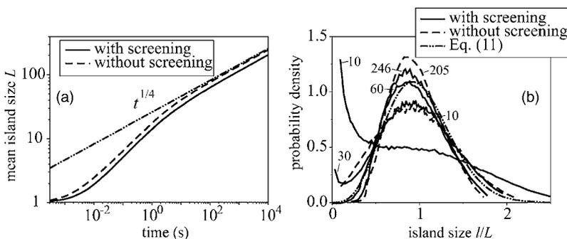
FIG. 6. Time dependence of the mean island size (a) and distribution functions (b) obtained by numerical solution of the Smoluchowski equations for the diffusion coefficient  $D_k=D_0/(1+k/k_0)$  and by the approximate formula (11).
