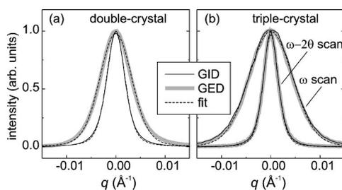
FIG. 2. Profiles of the 444 diffraction peaks in double-crystal (a) and triple-crystal (b) diffraction experiments.
