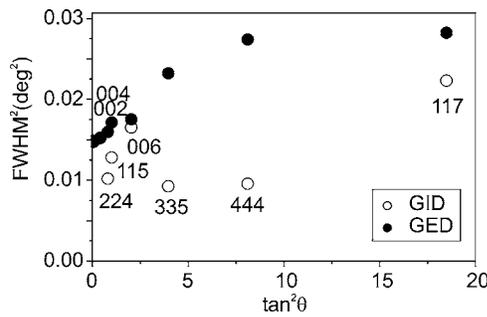
FIG. 1. Williamson-Hall plot for relaxed GaAs layer on Si(001). Open and full circles correspond to GID and GED geometries, respectively.
