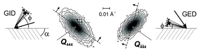
FIG. 3. Schemes of the GID and GED measurements and the reciprocal space maps in the two diffraction geometries. The broken lines perpendicular to the respective diffracted beam direction show the integration performed during a double-crystal measurement.
