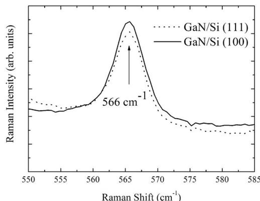
FIG. 4. Room temperature Raman spectra of GaN nanocolumns grown on both Si(001) and Si(111) substrates.
