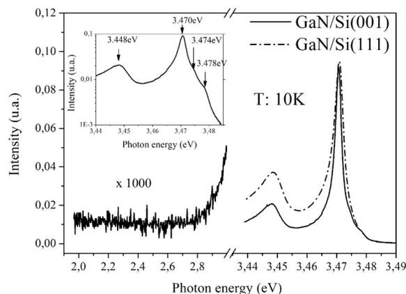
FIG. 3. Low temperature PL spectra of GaN nanocolumns grown on both Si(111) and Si(001) substrates. The inset shows in more detail the dominant near band edge emissions from the GaN nanocolumns grown on Si(001) substrate.
