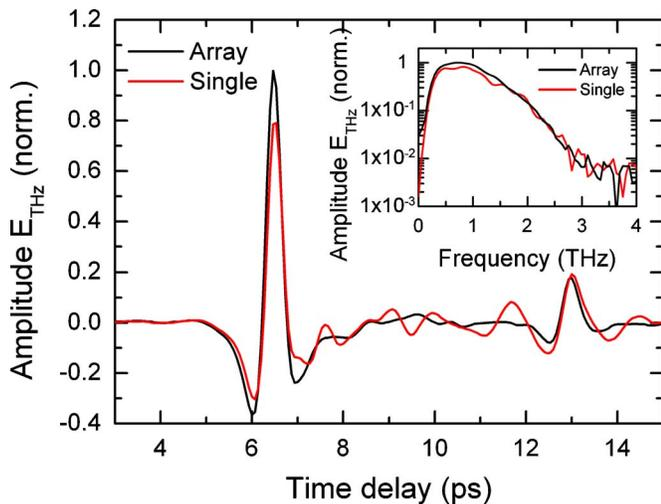
FIG. 2. (Color online) Time-resolved scans of terahertz pulse for array emitter (dark line) and single element (light line) and their respective spectra in inset.
