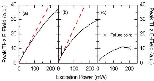
FIG. 4. (Color online) Saturation curve for (a) single element (focused optical spot, X marks failure point of the device), (b) reference excitation spot (spot size adjusted to maximize terahertz amplitude at low excitation power), and (c) array with large excitation spot compared to reference spot (spot size adjusted to maximize terahertz amplitude at high excitation power).
