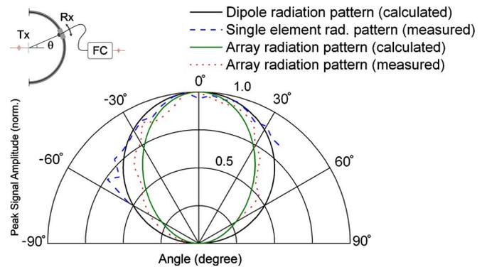
FIG. 3. (Color online) Calculated radiation pattern for dipole (black solid line) and measured single element radiation pattern (dashed line). Array radiation pattern calculated based on array theory (light solid line) and measurement (dotted). Inlay: experimental setup with fiber coupled and dispersion compensated (FC) receiver for radiation pattern measurement.
