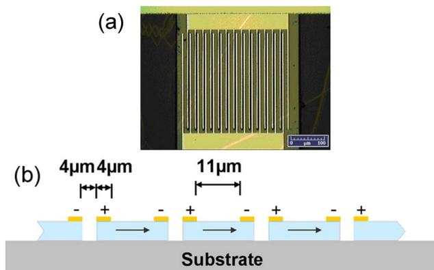
FIG. 1. (Color online) (a) Micrograph of terahertz array antenna device. (b) Cross-sectional view of terahertz antenna array.
