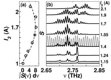
FIG. 3. (a) Integrated intensity and (b) longitudinal-mode spectra of sample B ( $L_3/L_1=3.7$ ,  $L_3+L_1=5360 \mu\text{m}$ ) for  $I_1=0.6 \text{ A}$  ( $I_c=2.3 \text{ A}$ ) and different values of  $I_3$ . The gray spectrum was calculated using Eq. (4). The dashed line in (a) is a guide to the eye.
