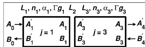
FIG. 1. Geometry of the TSCC laser.  $A_j$  and  $B_j$  denote the amplitude of the partial wave propagating to the right and left, respectively, on the left (unprimed) or right side (primed) of the interface  $j-1, j$ .
