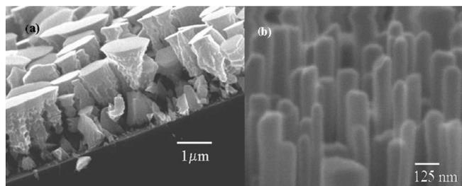
FIG. 1. (a) SEM image of pyramid-shaped InN nanocolumns grown close to the dissociation temperature (550 °C). (b) SEM image of InN nanocolumns grown at optimal temperature (475 °C).
