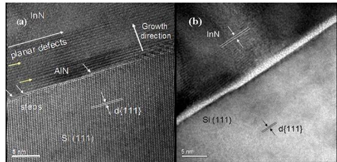
FIG. 3. (a) Cross-sectional HRTEM image of the AlN/Si(111) interface where step and planar defects are clearly seen. (b) Cross-sectional HRTEM image of the thin  $\text{Si}_x\text{N}_y$  layer developing at the interface between InN nanocolumns and the bare Si(111).
