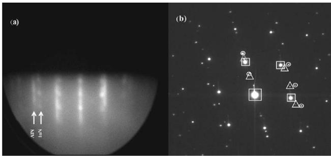
FIG. 2. (a) RHEED pattern of InN nanocolumns superimposed to the AlN-buffer one. (b) SAED image revealing three different diffraction patterns corresponding to Si(111) (squares), AlN buffer (circles), and InN nanocolumns (triangles).
