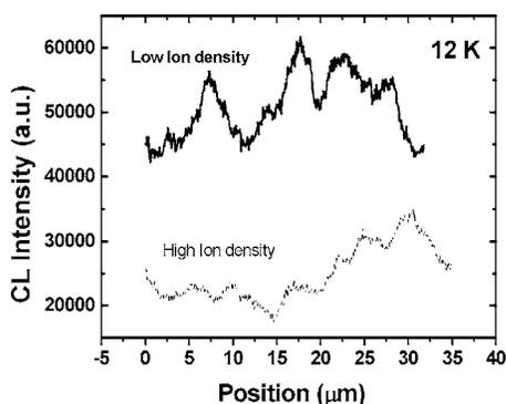
FIG. 3. Line scans of the low temperature (12 K) CL intensity of the GaInNAs QWs grown with a high (dashed line) and low (solid line) ion density. The detection energies were 0.933 and 0.943 eV, respectively.
