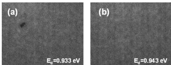
FIG. 2. Low temperature (12 K) CL mappings of the GaInNAs QWs grown with a high (a) and low (b) ion densities. The detection energies were 0.933 and 0.943 eV, respectively, which corresponds to the high-energy flank of the respective CL spectra.
