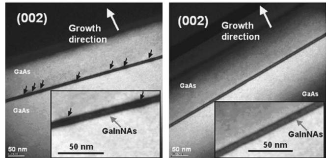
FIG. 6. Cross-sectional TEM image of the GaInNAs QWs grown without (a) and with (b) a deflecting magnetic field to reduce ion density, taken with diffraction vector  $g(002)$ , which is sensitive to the composition of the layer. The insets show in more detail the microstructure of the QWs. The black and white arrows indicate the compositional fluctuations and the growth direction, respectively.
