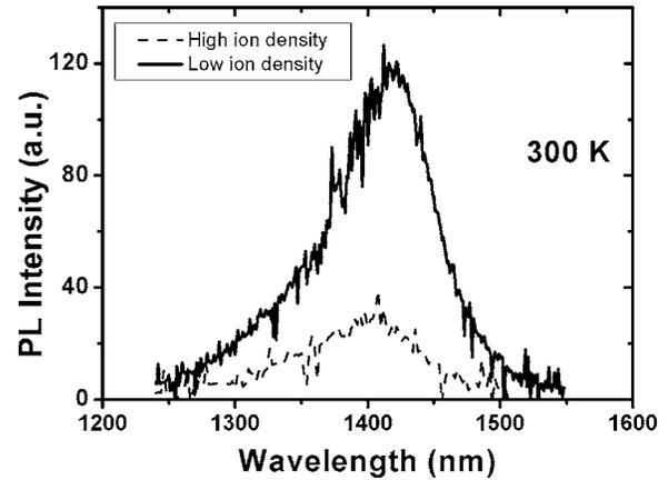
FIG. 1. Room temperature PL spectra of the GaInNAs QWs grown with high (dashed solid line) and low (black solid line) ion densities. The latter shows an improvement of PL intensity by a factor of 4.
