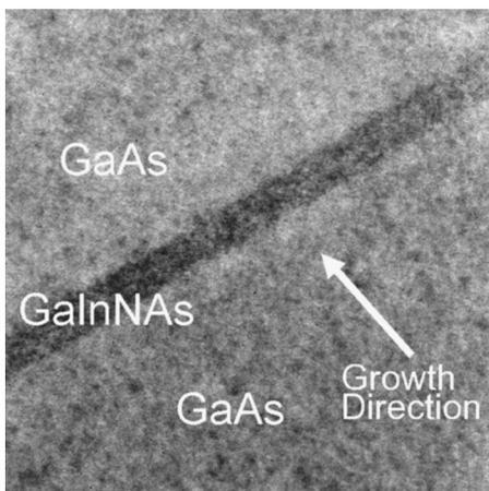
FIG. 7. High-resolution TEM picture of the GaInNAs QW grown with reduced ion density. Upper and lower interfaces are indistinguishable.
