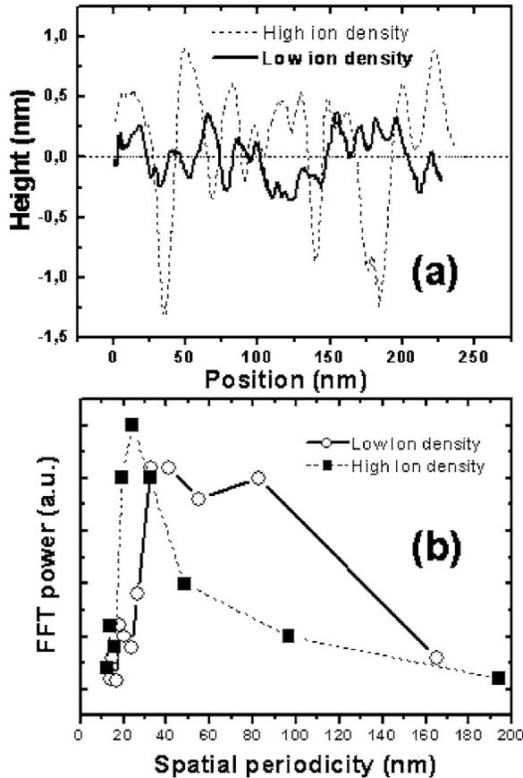
FIG. 5. (a) Surface line profiles of the GaInNAs epilayers, measured by AFM. The dashed (solid) line shows the epilayer grown with a high (low) ion density. (b) Fast-Fourier transform of the average of several cross-sectional profiles of the epilayers grown with a high (filled squares) and a low (hollow circles) ion density. Lines are interpolations between data points.
