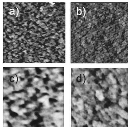
FIG. 4. AFM images of the GaInNAs epilayers, grown with a high [(a),(c)] and a low [(b),(d)] ion density. (a) and (b) scans are  $500 \text{ nm} \times 500 \text{ nm}$  with a vertical scale of 3 nm. (c) and (d) scans are  $180 \text{ nm} \times 180 \text{ nm}$  with a vertical scale of 5 nm.
