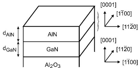
FIG. 1. Schematic of layered system. A (0001)-oriented hexagonal AIN/GaN bilayer is placed on a trigonal Al<sub>2</sub>O<sub>3</sub>(0001) substrate. The crystal orientation relationship is indicated on the right-hand side. The thickness of the AIN and GaN layers is  $d_{\text{AIN}}$  and  $d_{\text{GaN}}$ , respectively.
