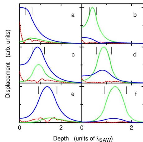
FIG. 5. (Color online) Depth profile of the displacement of particles of the medium at the points marked “a”–“f” of the lowest two modes around  $d_{GaN}/\lambda_{SAW}=0.5$  in Fig. 3. The dashed, dotted, and solid curves correspond to the longitudinal displacement  $u_1$  and transversal displacements  $u_2$  and  $u_3$  in the in-plane and depth directions, respectively. The bars indicate the location of the heterointerfaces.
