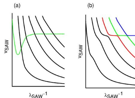
FIG. 7. (Color online) Interpretation of the dispersion in a system consisting of an AlN/GaN bilayer and a substrate in terms of mode coupling. We assume two kinds of acoustic modes whose dispersion behaves as schematically shown in (a) when they are decoupled. A coupling between the modes shown by the dotted and solid curves in (a) gives rise to anticrossings, as illustrated in (b).
