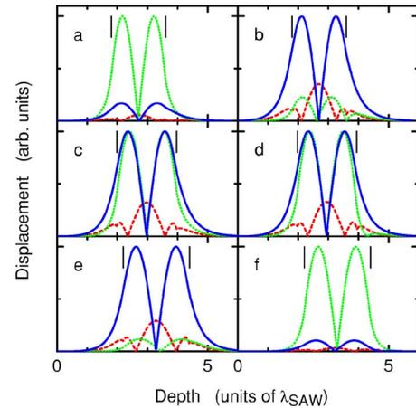
FIG. 4. (Color online) Depth profile of the displacement of particles of the medium at the points marked “a”–“f” of the third and fourth modes around  $d_{GaN}/\lambda_{SAW}=2$  in Fig. 3. The dashed, dotted, and solid curves correspond to the longitudinal displacement  $u_1$  and transversal displacements  $u_2$  and  $u_3$  in the in-plane and depth directions, respectively. The bars indicate the location of the heterointerfaces.
