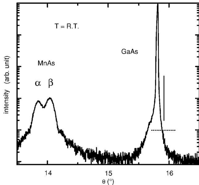
FIG. 5. X-ray diffraction curve of the unpatterned MnAs/GaAs structure at room temperature. The three peaks from left to right are associated with the  $[1\bar{1}00]$  reflection of  $\alpha$ -MnAs,  $[020]$  reflection of  $\beta$ -MnAs, and  $[002]$  reflection of GaAs. The peak position expected for the  $[1\bar{1}01]$  reflection is indicated by the vertical bar. A prediction of the peak amplitude when the fraction of type- $B_1$  MnAs is 3.5% is shown by the horizontal dotted line.
