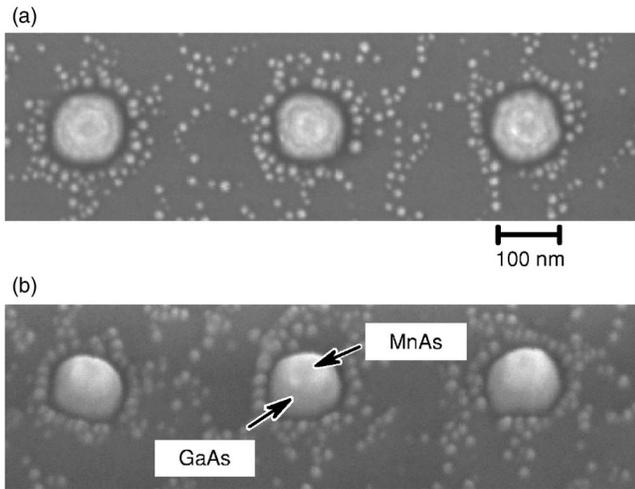
FIG. 2. Scanning-electron micrographs of MnAs dots on a GaAs substrate. Top and glancing-angle views are shown in (a) and (b), respectively. MnAs dots are placed on top of GaAs pillars.
