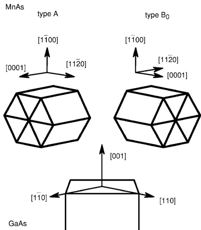
FIG. 1. Crystal orientation relationship for a MnAs layer grown on a GaAs(001) substrate. The *c* axis of hexagonal MnAs is along the [1 $\bar{1}$ 0] and [110] directions of GaAs for the type-*A* and type-*B*<sub>0</sub> orientations, respectively.
