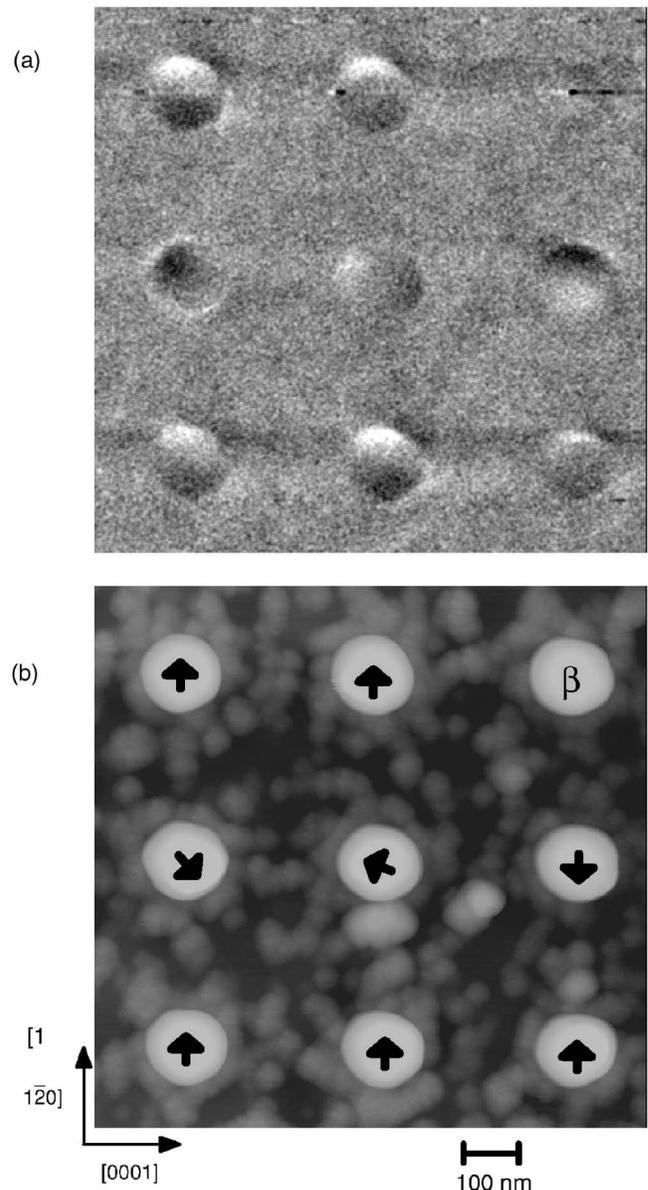
FIG. 3. (a) Magnetic- and (b) atomic-force micrographs of MnAs dots on a GaAs(001) substrate. The arrows in (b) indicate the direction of the magnetic moment in ferromagnetic dots. A nonmagnetic dot consisting of  $\beta$ -MnAs is indicated by " $\beta$ ." The magnetic easy axis of the MnAs layer is along the  $[1\bar{1}20]$  direction.
