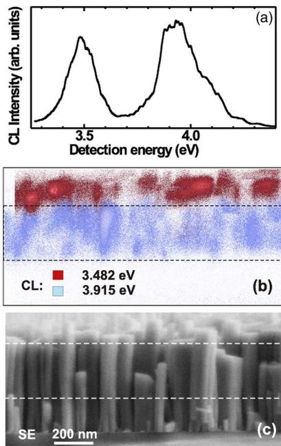
FIG. 2. (Color online) (a) CL spectrum of a large number of GaN/(Al,Ga)N nanocolumns containing 4.2-nm-thick QDisks. (b) Superimposed CL images differing in the detection energy. The dark and bright colored images correspond to CL detection energies of 3.482 and 3.915 eV, respectively. (c) SEM image of the GaN/(Al,Ga)N nanocolumns investigated by CL in (a) and (b). The spectrum and images have been obtained at 6 K.
