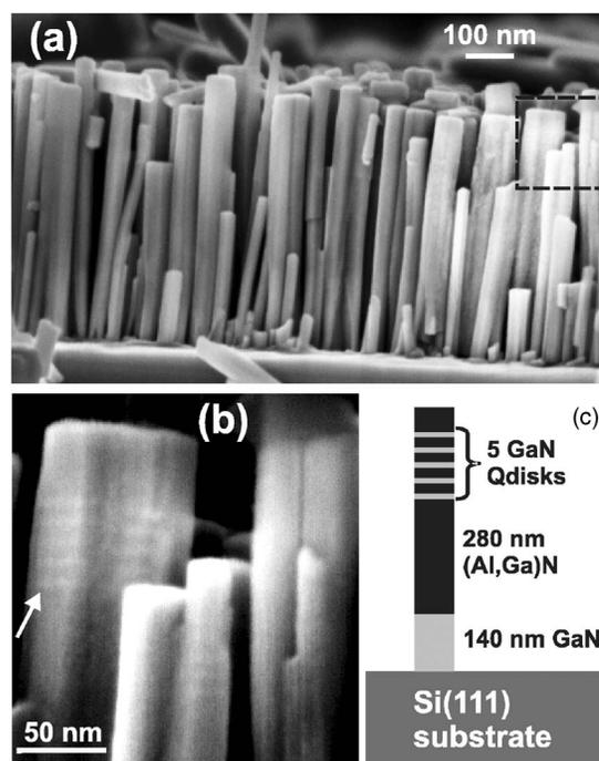
FIG. 1. (a) SEM image of GaN/(Al,Ga)N nanocolumns with 3-nm-thick GaN QDisks. (b) Magnified SEM image of the sample region marked by the dashed rectangle in (a). The arrow points to the 3-nm-thick QDisks. (c) Schematic diagram of the columnar heterostructure.
