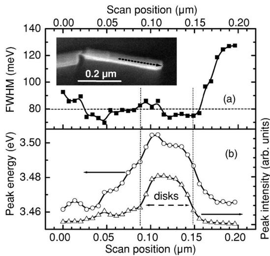
FIG. 4. (a) FWHM and (b) peak energy (circles) and peak intensity (triangles) of CL spectra measured along a line [dashed arrow in the inset of (a)] crossing the QDisk region of a single nanocolumn at 6 K. The dashed vertical lines mark the QDisk region. Inset of (a): SEM image of the GaN/(Al,Ga)N nanocolumn.
