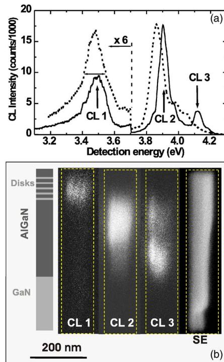
FIG. 3. (Color online) (a) CL spectra of two single GaN/(Al,Ga)N nanocolumns at 6 K. (b) CL images and SE image of the single nanocolumn represented by the solid line in (a) at 6 K. The detection energies used for CL imaging are marked by arrows in (a).
