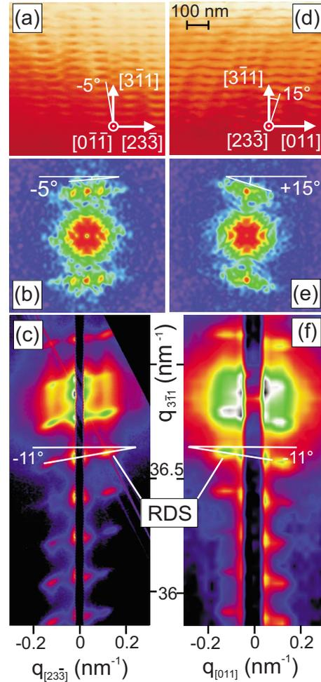
FIG. 2. (Color online) Vertical stack with 135 ML spacer thickness. Bright field XTEM images containing the  $[011]$  (a) and  $[23\bar{3}]$  (d) directions. Corresponding XTEM power spectra (b, e) and HRXRD reciprocal space maps (c, f) were used to deduce the angles of inclined inheritance,  $\alpha_{011}$  and  $\alpha_{23\bar{3}}$ , of the QD stacking in the corresponding projections.
