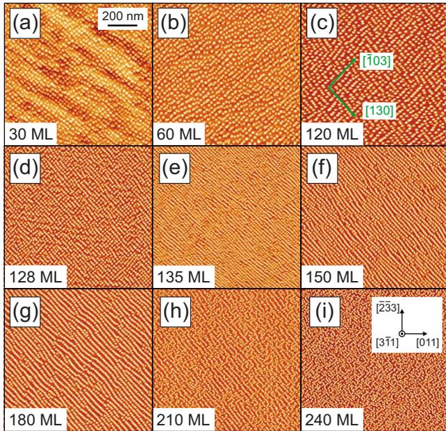
FIG. 1. (Color online) Atomic force micrographs of the topmost surface for various (In,Ga)As/GaAs QD SLs grown on GaAs(311)B. The thickness of the GaAs spacer layers between succeeding QD layers varies between 30 and 240 ML. The green arrows mark the planar [130] and  $[\bar{1}03]$  directions.
