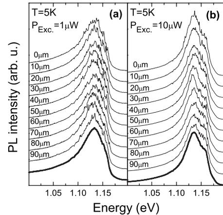
FIG. 2. Low temperature  $\mu$ -PL spectra measured along a line at the excitation powers of (a) 1  $\mu$ W and (b) 10  $\mu$ W.
