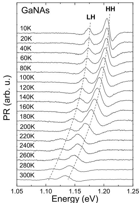
FIG. 4. Temperature dependence of PR spectra for GaNAs layer.
