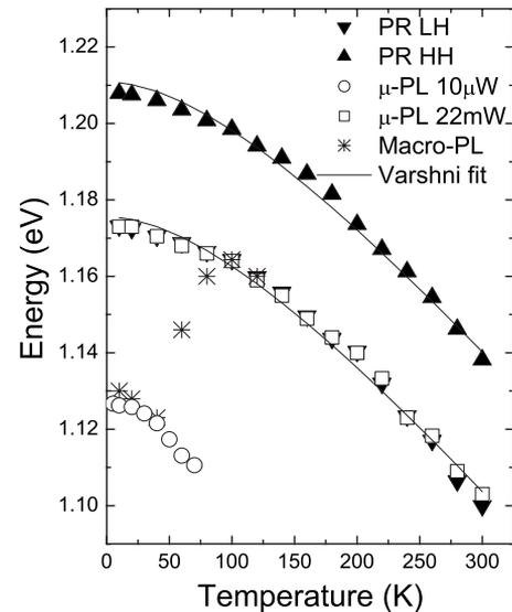
FIG. 5. Temperature dependence of LH (▼) and HH (▲) transitions in GaNAs layer extracted from PR spectra and the energy of PL peak (i.e., the envelope of PL band). Varshni parameters:  $\alpha^{\text{LH}} = \alpha^{\text{HH}} = 0.42 \text{ meV/K}$  and  $\beta^{\text{LH}} = \beta^{\text{HH}} = 230 \text{ K}$ .
