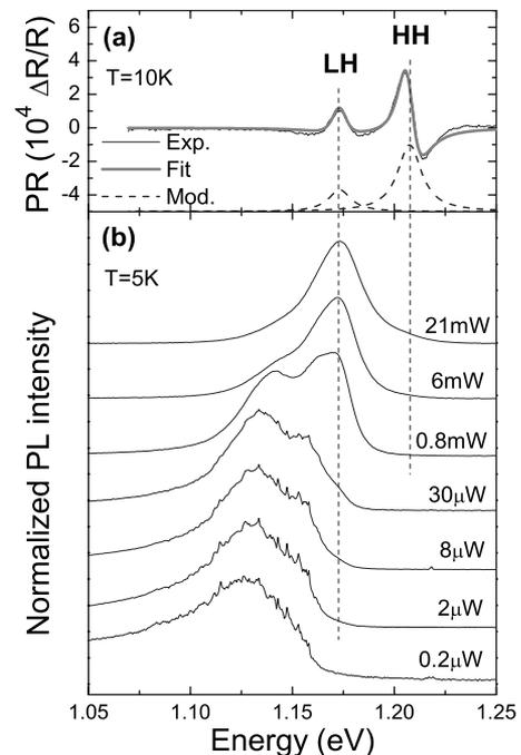
FIG. 1. (a) PR and (b)  $\mu$ -PL spectra for GaNAs layer measured at low temperatures.
