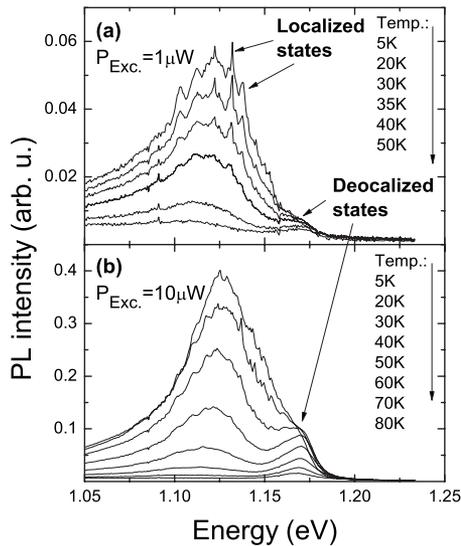
FIG. 3. Temperature dependence of  $\mu$ -PL spectra measured at the excitation powers of (a)  $1 \mu\text{W}$  and (b)  $10 \mu\text{W}$ .
