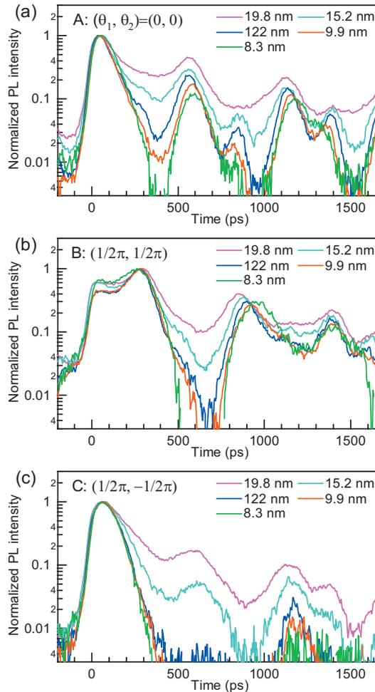
FIG. 2. (Color) [(a)–(c)] Normalized time traces for the 8.3, 9.9, 12.2, 15.2, and 19.8 nm QWs under a standing SAW with  $(\theta_1, \theta_2) = (0, 0)$ ,  $(1/2\pi, 1/2\pi)$ , and  $(1/2\pi, -1/2\pi)$ , respectively. The PL intensity was selectively integrated at the photon energies of 1.527, 1.537, 1.549, 1.569, and 1.585 eV.
