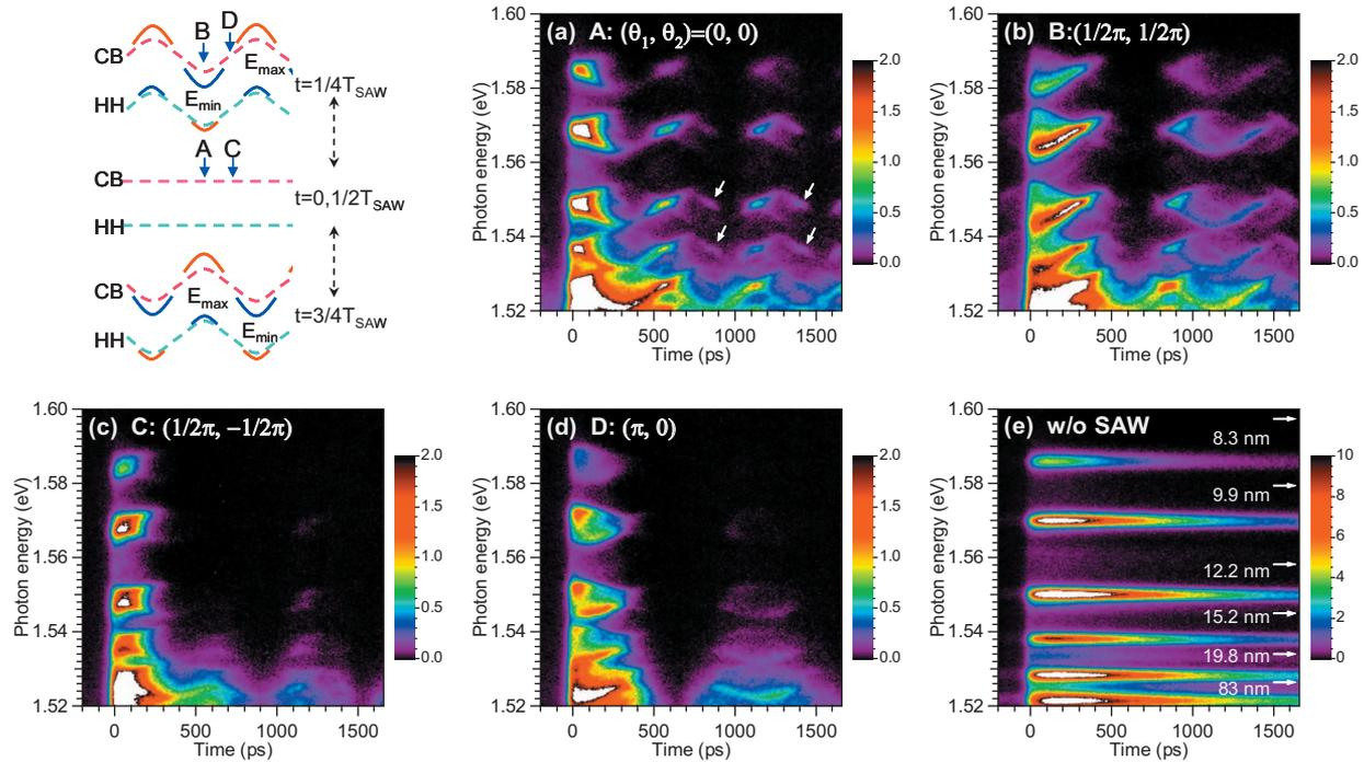
FIG. 1. (Color) An inset illustration schematically shows changes in the band structure modulated by a standing SAW. [(a)–(d)] Time-resolved PL spectra measured at the same position under the standing SAW with different phases of  $(\theta_1, \theta_2) = (0, 0)$ ,  $(1/2\pi, 1/2\pi)$ ,  $(1/2\pi, -1/2\pi)$ , and  $(\pi, 0)$ , respectively. (e) Corresponding spectrum in the absence of a SAW.
